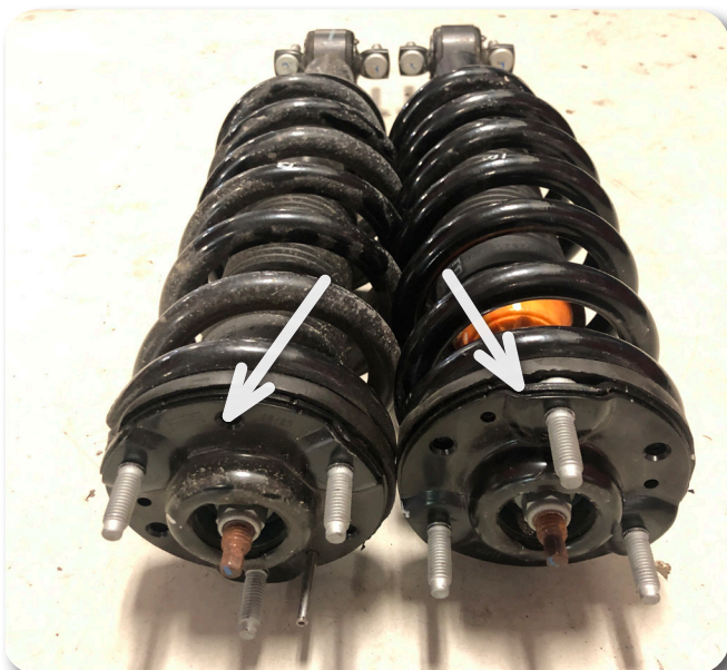
Figure 18 (Strut on the right has the top hat rotated 180 degrees, strut on the left is stock orientation with the bar pin angle the same)
