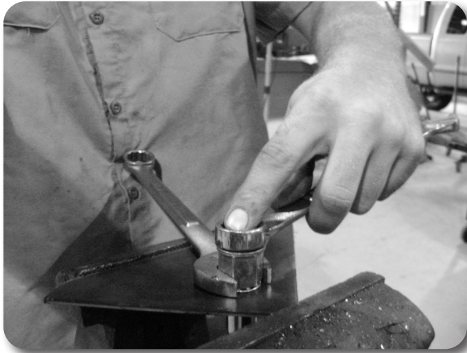
Figure 4 - 1/2" Rivet Nut shown
