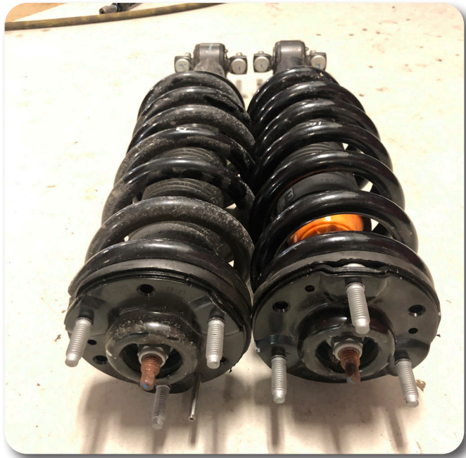
Figure 11B (Strut on the right has the top hat rotated 180 degrees, strut on the left is stock orientation with the bar pin angle the same)
