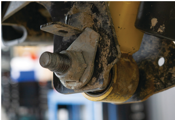
Fig. 25: Loosen the lower mounting bolt.
