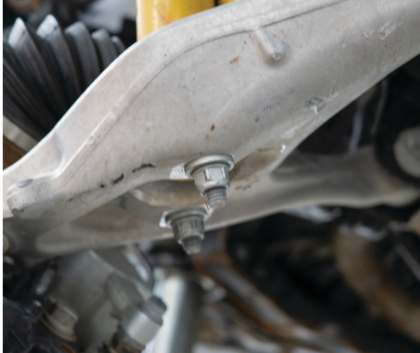
Fig. 9: Take off the bar-pin bolts.
