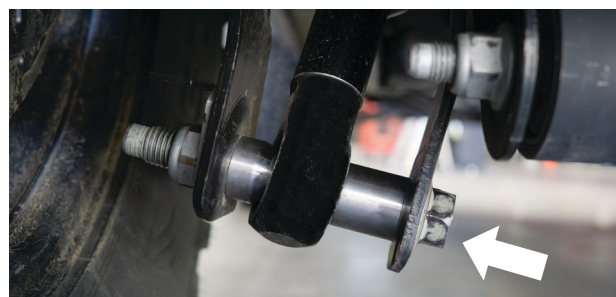
Fig. 29: The larger spacer mounts on the inboard side of the eyelet.
