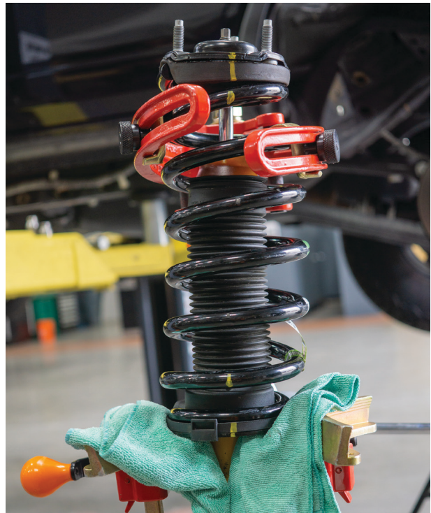
Fig. 11: Use a professional spring compressor.
