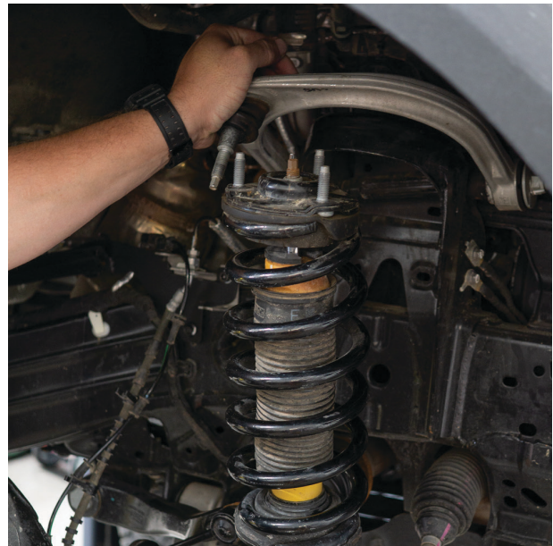
Fig. 8: Free the coil-over from the coil bucket.
