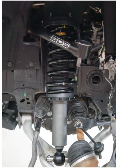
Fig. 16: Align marks on the coil bucket and top hat.
