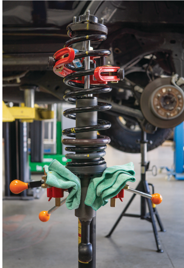
Fig. 27: Align the marked top hat, spring, and eyelet.
