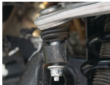
Fig. 5: Separate the UCA from the upright.
