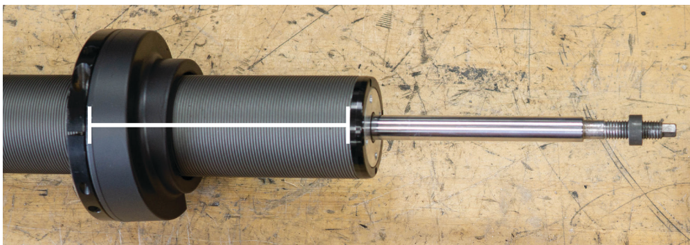
Fig. 14: Measure from the preload ring to the bottom of the bearing cap.
