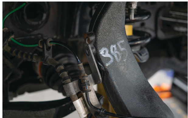
Fig. 1: Disconnect brake line bracket.
