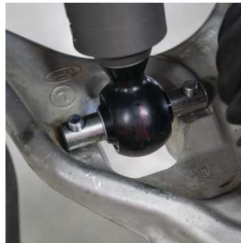
Fig. 18: Fasten the bar-pin bolts.
