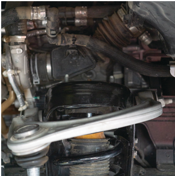
Fig. 7: DO NOT remove the center nut.
