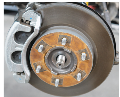
Fig. 4: Push the axle shank flush.
