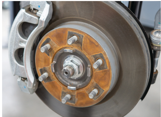
Fig. 20: Fasten the axle nut.
