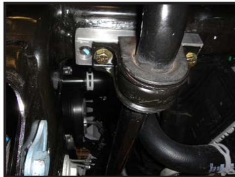
**15.** Using a 13mm socket/wrench loosen the brake line bracket on the coil bucket. Push it down and slightly bend it rearward. [Torque to factory spec] (FIGURE 15 AND 16)
