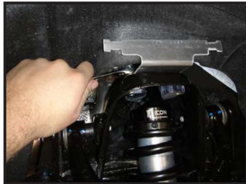
**13.** The bottom spacers on the coilover assembly push the coilover away from the CV boot. Installing these spacers backwards will cause the CV boot to rub the rod end. Reuse the factory lower bolt and a 21mm socket/wrench to fasten. [Torque to factory spec] (FIGURE 12)
