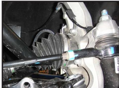
**19.** Reconnect the tie rod to the knuckle using a 21mm socket/wrench. [Torque to factory spec] (FIGURE 20)
