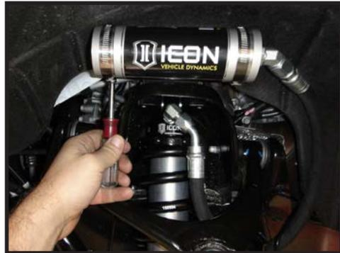
**15.** Mount the reservoir to the reservoir mount using the supplied hose clamps and a 5/16" nut driver. (FIGURE 13)
