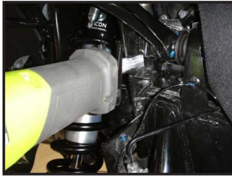
**12.** Slide the ICON coilover assembly into position and fasten it using the supplied 3/8" bolts and washers with a 9/16" socket/wrench [Torque to 30ft-lbs]. Make sure the reservoir hose is pointing toward the rear of the truck. (FIGURE 10) Place the reservoir mount on top of the coil bucket before as shown. (FIGURE 11)
