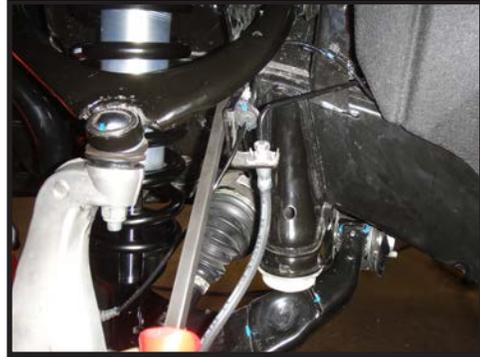
**16.** Reattach the UCA to the knuckle using a 18mm socket/wrench. [Torque to factory spec] (FIGURE 17)
