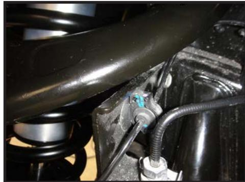
**17.** Verify that brake line tab, UCA and reservoir hose do not make contact at full droop. Failure to route the hose properly can cause damage to the hose which is NOT covered under warranty. (FIGURE 18)
