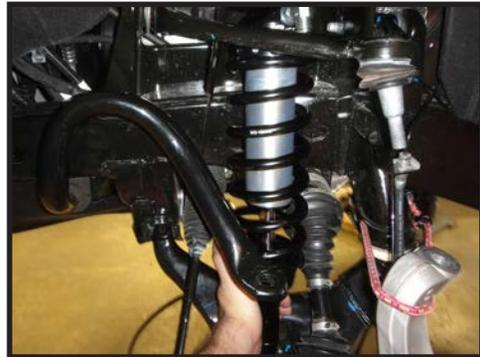
**10.** With the OEM coilover removed, sway bar removed, and UCA free from the knuckle, sand the lower shock tab as shown. Failure to sand this section will allow the CV boot to rub at full droop and full steering lock. Be careful not to hit the CV boot. (FIGURE 7 AND 8)
