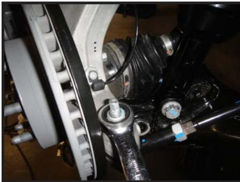
**9.** Remove upper ball joint nut to allow room for coilover removal, use a 21mm socket/wrench and a 2lb sledge on the knuckle to unseat taper. Tie up the neck of the knuckle so the CV joints do not over extend. (FIGURE 5 AND 6)
