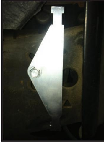
**5.** Using a 9/16" socket, install the supplied self tapping bolt (605144) into the previously drilled hole to create new threads. Remove bolt.
