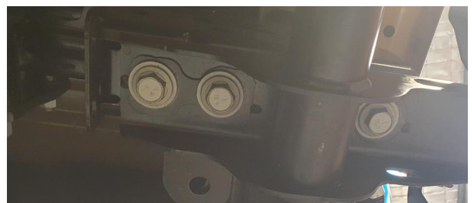
Above: Showing the 3x M16 bolts on the heavy-duty tow pack
