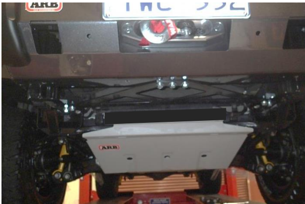
Fit front panel to vehicle
