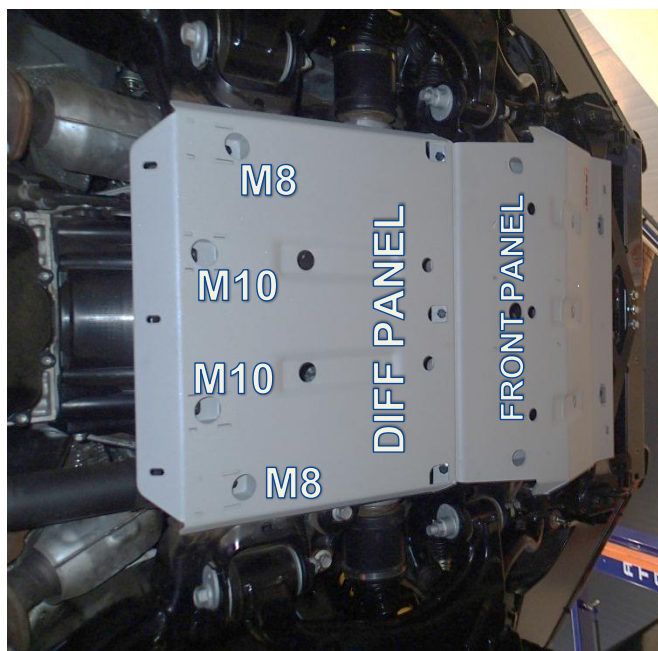
Fit differential panel to vehicle
