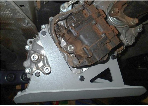
Transfer case panel rear side
