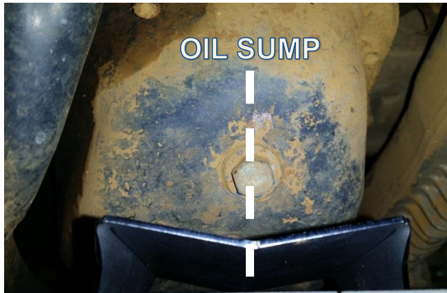
Align oil drainage bracket with sump plug bolt
