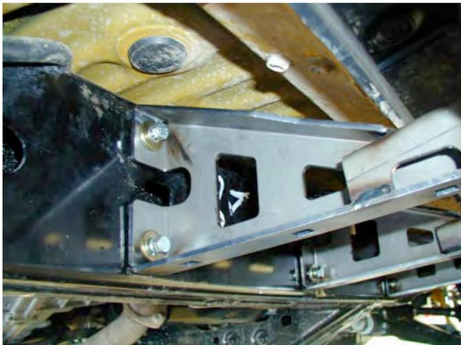
2. With the help of another person, carefully lift the rocker rails up to the chassis. Fix in place using the M8 x 25mm bolts, M8 spring washers and M8 x 24mm flat washers.
