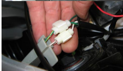
Indicator lamp wiring
