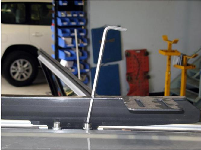
9. Position the mounting rail carefully on the roof and fix in place using the M8 x 30mm bolts prepared earlier.
