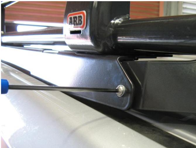
3. Attach the deflector to the mounting brackets using the remaining M6 cap screws and flat washers. **Tighten all bolts to specified torque.**
