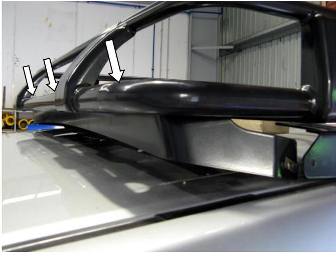
2. Attach the wind deflector to the roof cage along the top using the M6 x 16mm dome head cap screws and M6 flat washers.
