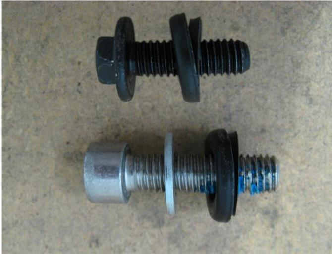
4. Remove the cap and rubber grommet from the bolts removed from the roof.
