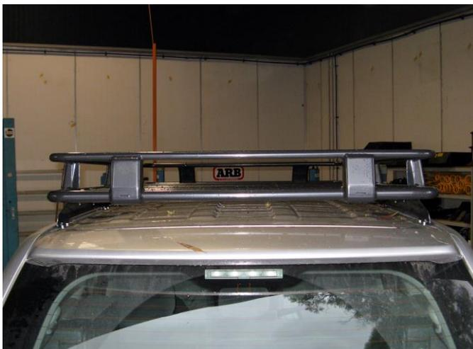
11. With assistance, carefully place the roof cage on the vehicle so that all mounting holes are aligned.
