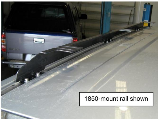
10. When all bolts have been fitted centralise the mounting rails and **fully tighten the bolts to specified**
