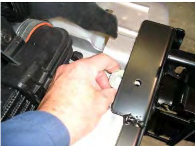
**29. Fit packer in between mount assembly and vehicle crossmember and align with the two holes.**
