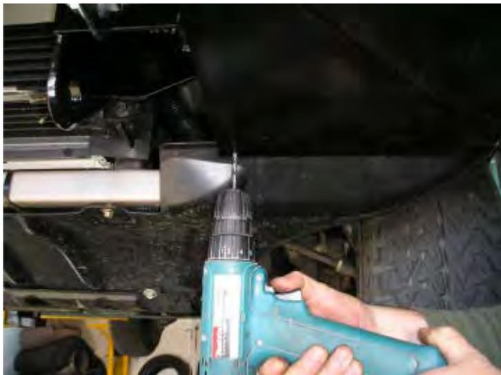
**63. Drill a 6mm hole into plastic vehicle splash pan using hole in wing panel as a template.**
