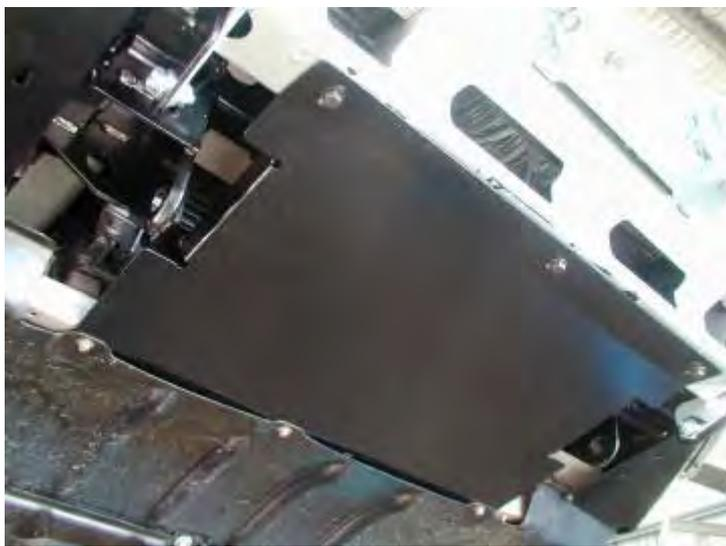
**67. Fit front of air deflector to underside of bar using black 8mm hardware.**
