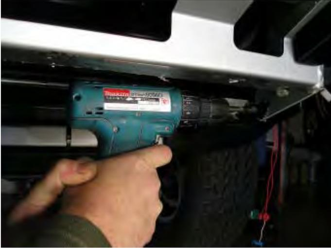
**58. Once the bar is secured to vehicle, using holes in lower section of bar as a template, drill 10mm holes through mounting assembly and fix using 10mm hardware.
