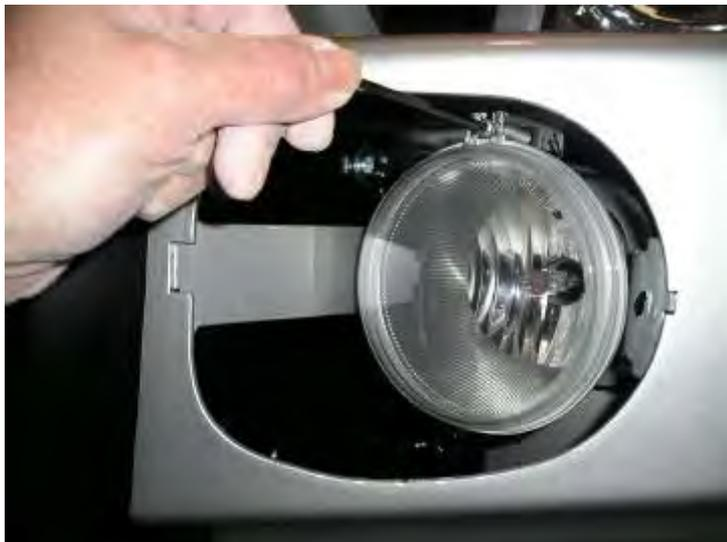
**76. When light is fitted to bracket refit adjuster screw then reset light alignment.**
