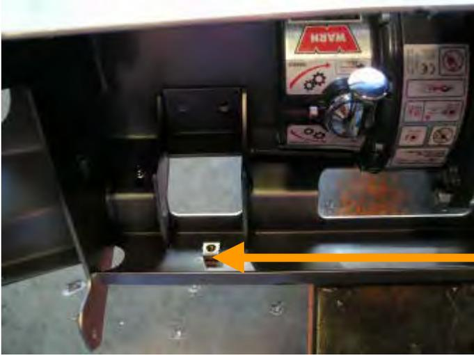
**54. Fit M8 caged nuts ( 3 OF ) into lower section of bar.**
