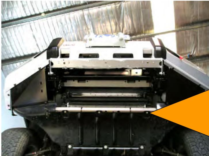
**67. Undo the three 6mm bolts as per photo so air deflector pan can fit in between.**
