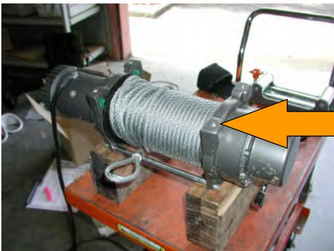
**48. To fit winch into bar you must pack winch up on a bench to enable you to lower bar down on winch, then fit four 3/8" square nuts into winch lugs.**
