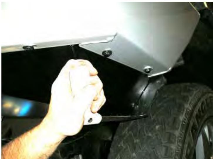
**65. After under wing panels are all bolted up, using a key hole saw etc, cut off the plastic under guard which protrudes past the panels.**
