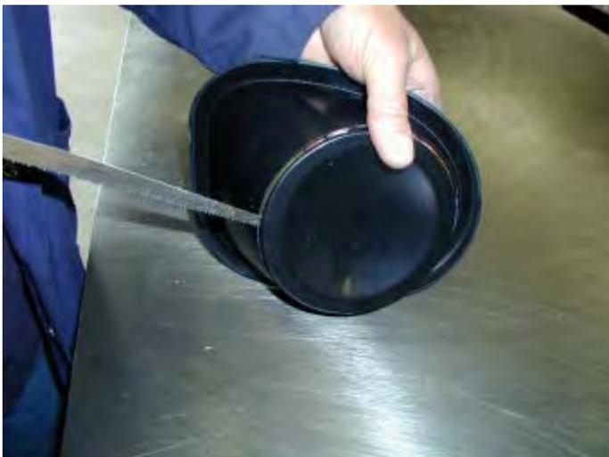
**69. If no fog lights are not going to be fitted, fit light surround to bar as is. If fog lights are going to be fitted, cut out rear of surround using a key hole saw and remove rough edges with a file.**
