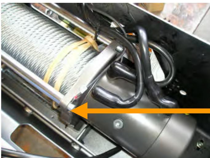
**52. Cable tie power cables clear of sharp edges and all moving parts.**
