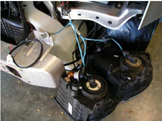
**5. After removing headlights from vehicle, remove some of the blue insulating tape from vehicle indicator and parking looms to expose wiring to be able to fit connectors.**
