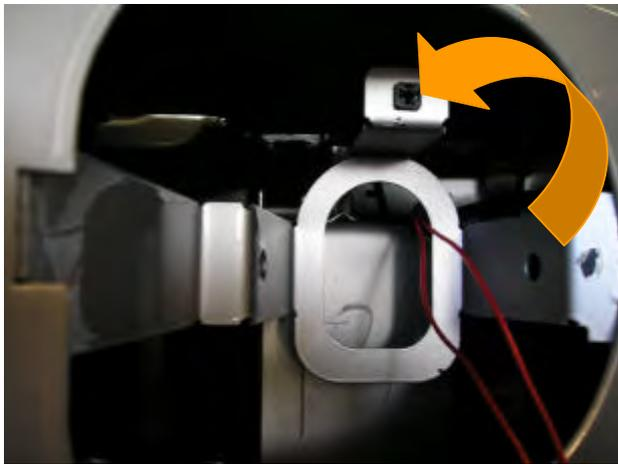
**72. If fitting fog lights back into vehicle, pull extended loom through fog light mounting bracket and refit black plastic grommets back into square hole.**
