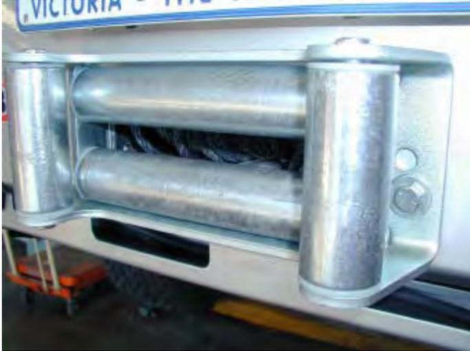
**49. Lower bar down over winch, line up top holes first and secure using 3/8" hardware (1 1/2" x 3/8" bolts) flat and spring washers.**
