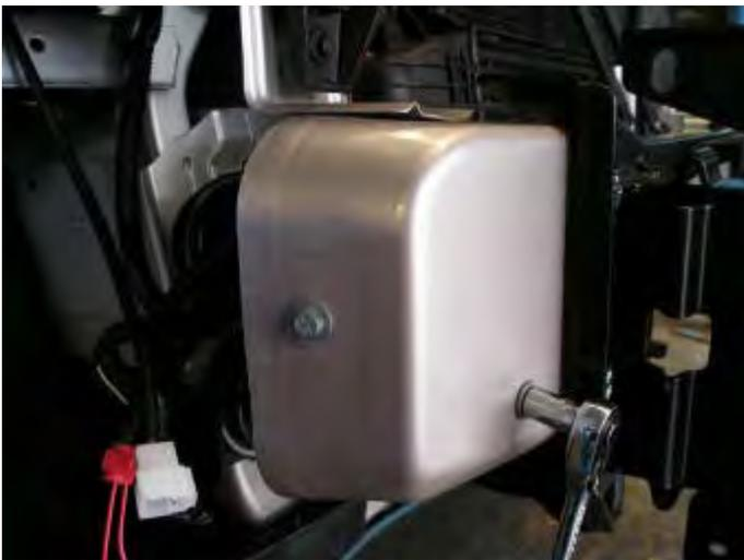
**38. Refit alarm device at this stage.**
