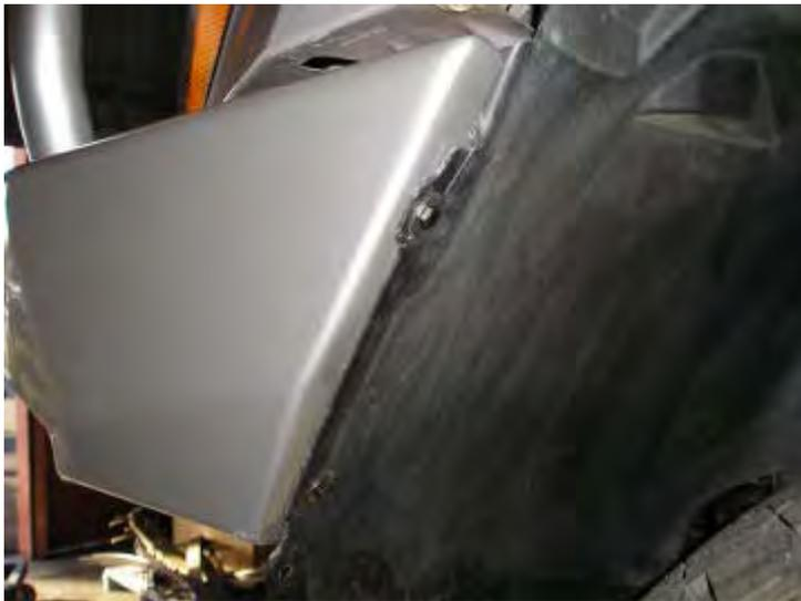
**59. Using 6mm hardware, secure plastic inner guard to top hole in bar.
