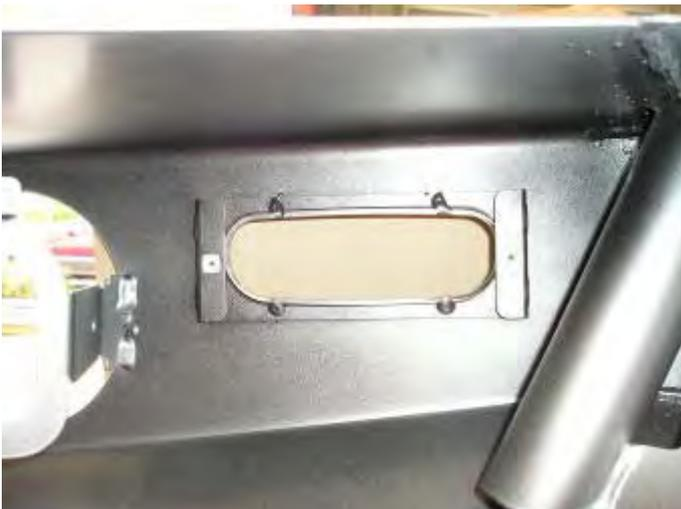
**39. Fit nylon grommets into square holes to mount indicator / parker lamps**
