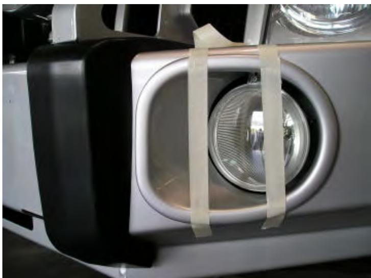
**77. Follow steps to fit light housing to bar same as paragraph 71. NB. Photo shows silicon applied around fog light cutout.**
