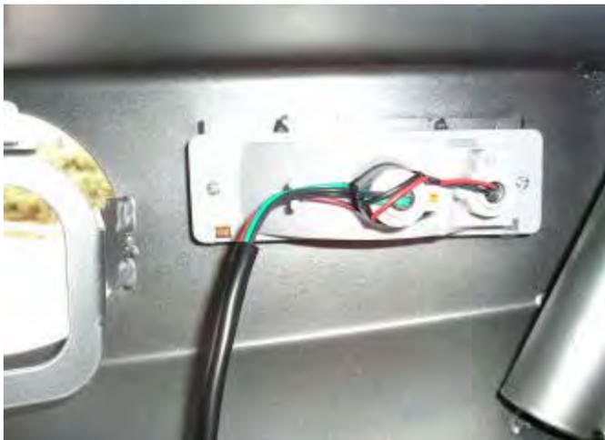
**40. Remove the fastening screws and nuts supplied with the turn signal/clearance lamps and replace these with the four screws provided in the kit. Fasten the lamps to the bar as shown.**
