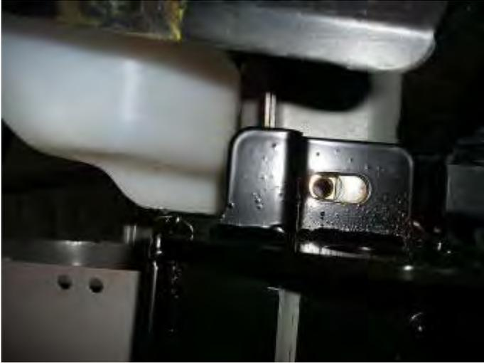
**22. As viewed from underneath on LHS of vehicle, align rear hole of mount assembly to previously fitted captive nut channel, secure using M10 bolt x 30mm SEMS ( Bolt, Spring and Flat Washer ASSY. )**
