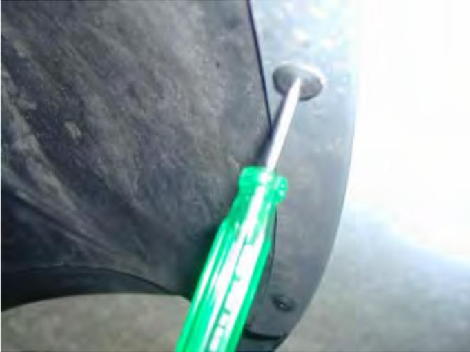
**3. To remove bumper bar where the inner guard is attached, push plastic pin inward , then pull out plastic retainer clip. Remove fog lights and fog light adjuster and the black plastic grommets from bumper.**
