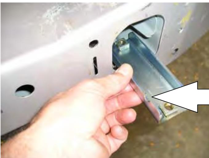
**14. Fit M10 caged nuts into channel ( channels are L/RHS ) then fit channels inside of chassis rails**
