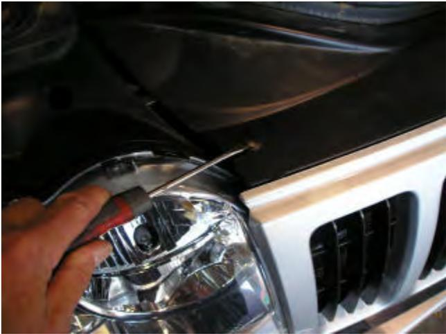
**1. Remove grille from vehicle by removing all plastic clips**
