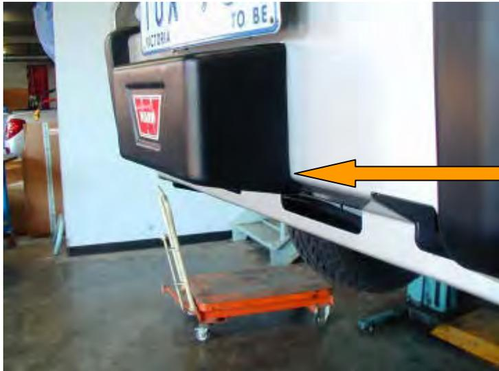
**79. The Warn roller fairlead cover must be fitted to roller fairlead when winch is not in use due to protruding sharp edges legislation.**
