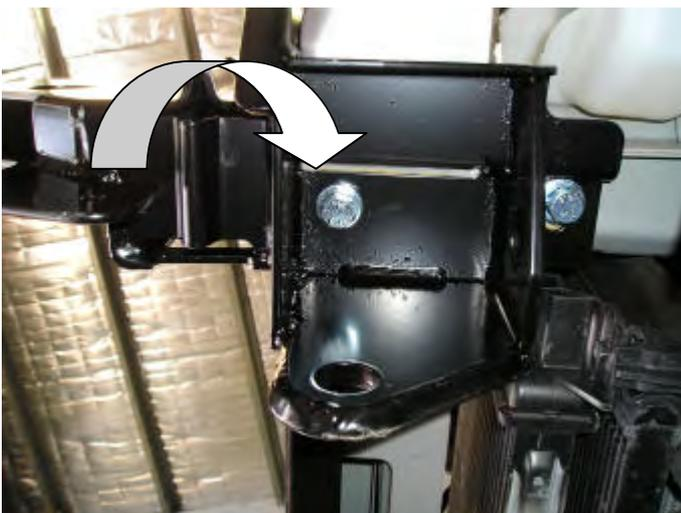
**25. Using a 10mm drill bit, drill hole through chassis rail, using hole in mount as a template. Be careful not to drill into the nut in captive nut channel.**
