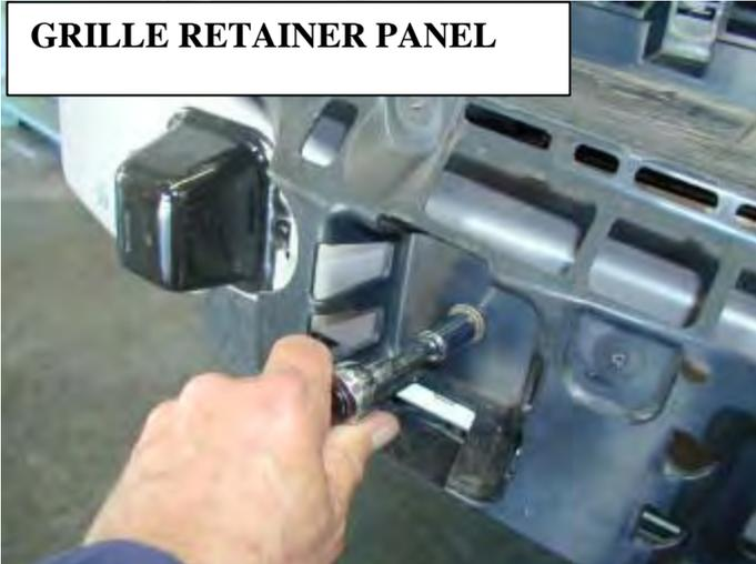
**2. Remove lower plastic grille retainer panel from vehicle and put aside, as this panel will have to be modified later.**
