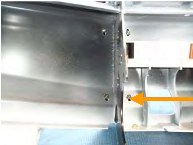
**47. Fit buffers to bar using 6mm flange nuts.**
