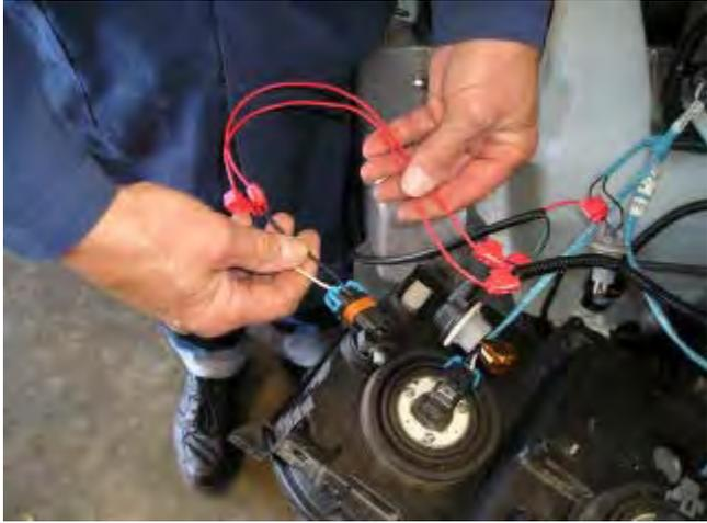
**10. Scotch lock the red wire in between the fog light loom making sure the colour code matches.**
