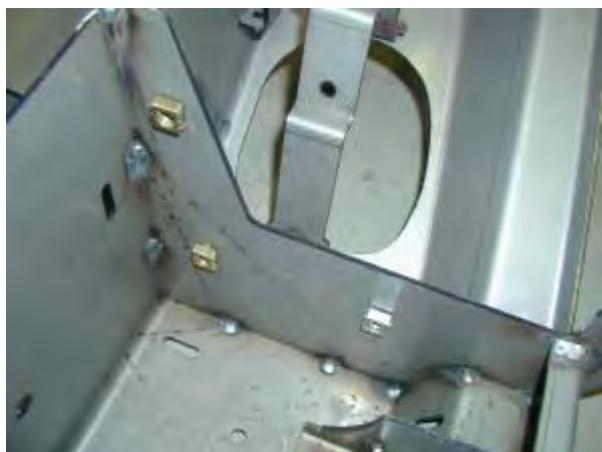
**41. Fit M10 caged nuts to inside of mounting face of bar.**
