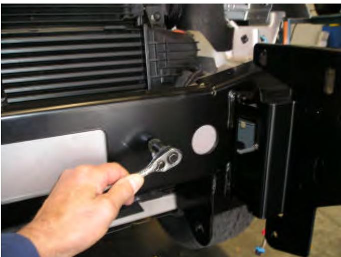
19. Lift chassis mount assembly onto vehicle crossmember.
