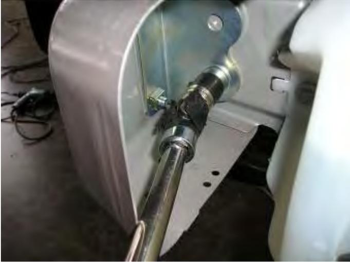
**37. Tighten this 12mm bolt each side using universal joint and 1/2" drive extension.**
