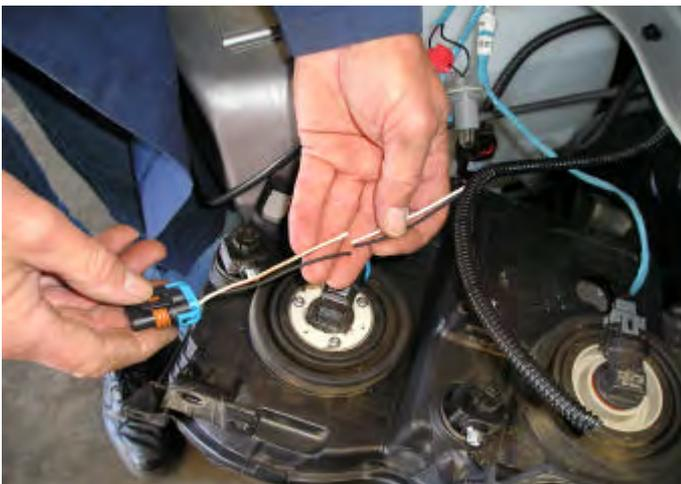
**8 . To refit fog lights to bar, the loom must be extended.**
