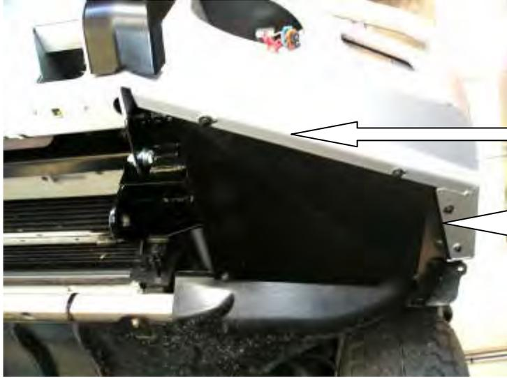
**62. Fit panel on top of wing returns and secure using 6mm hardware.**
