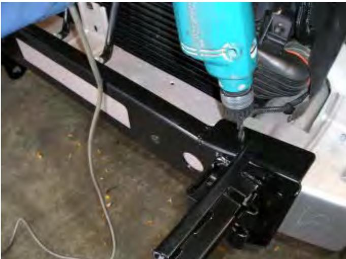
**28. Also drill through top of mount into vehicle crossmember, making sure that you are drilling perpendicular.**
