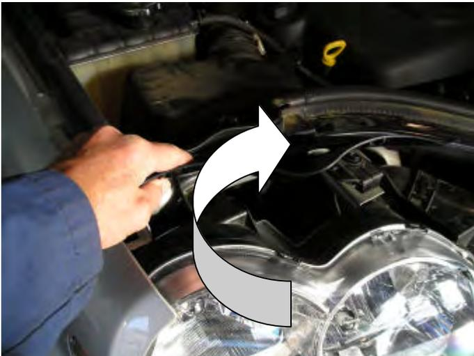
**4. To remove headlights from vehicle for ease of joining indicator looms and extending fog light looms, firstly lift plastic cover from above headlight and undo one plastic retaining clip and three 6mm bolts, then remove headlights.**
