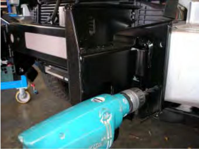
**27. Using holes in chassis mount assembly as a template, drill through crossmember on both sides using 10mm drill bit.**
