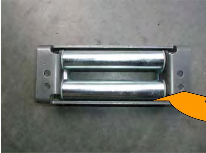
**46. Drill 12mm holes under existing holes 25mm lower down the same pitch as existing holes, these will be the holes used to bolt roller fairlead to bar.**
