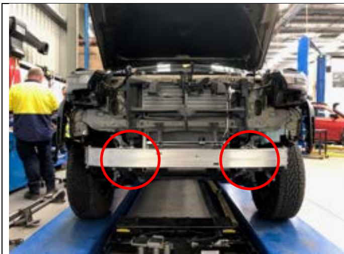
OEM bumper support bracket
