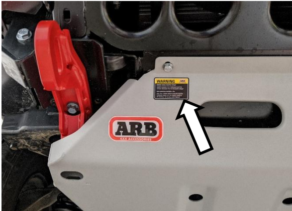
Label position with ARB Under Vehicle Protection in conjunction with ARB bull bar
