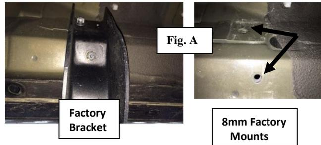
**Step 2:** Starting with the driver's side, lift step up into position aligning the step bracket with the 8mm OE mounts. (Fig. B)
