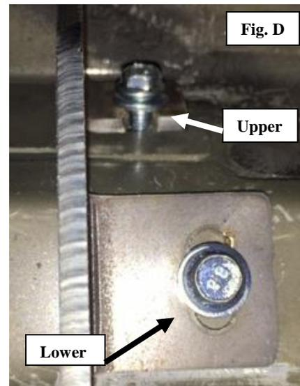
**Step 5:** Repeat steps 2-4 with the passenger side. **NOTE: Periodically check all hardware for tightness to insure longevity and safety of your steps.**
