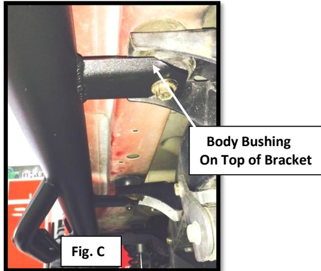
**Step 4:** Next, install the front body bolt and bushing and loosely tighten... **NOTE:** *Be sure the round opening in the step bracket fits around the upper body bushing and set s flush with body mount not to pinch the bushing. Fig. D*
