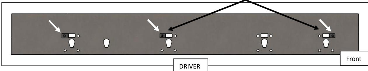
**Step 3:** Next, install the step aligning the brackets to the upper clips using the 3/8"x1" Hex bolt, 3/8" USS Flat washer for the upper attachment and the 3/8"x 1 1/2" carriage bolt 3/8" Hex nut and 3/8" USS washer for the lower attachment. Leave loose for now. **NOTE: The carriage bolts will start from the outside of the body, the nut and washer will be only visible from underneath the vehicle.**
