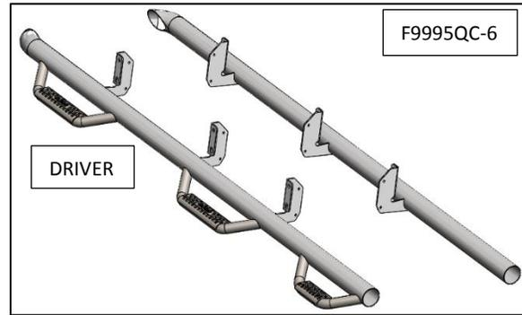
**Step 2:** Starting with the Driver side, locate the holes for the upper mounts (x3) and install the supplied (x2) 3/8" clips in each position. **NOTE: There will be four attachment points for the Quad Cab and five for the Crew Cab. Only three will be used for the installation. See below for your cab configuration.**
