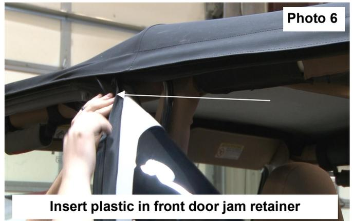
**Insert plastic in front door jam retainer**
