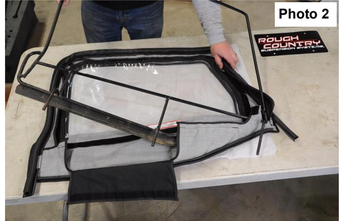
4. The rear upper corner will be the last part to pull over the frame work. There is a tab sewn into the fabric to help you pull the fabric over the frame work. Once the frame is inside the fabric make sure all panels and loop flaps are pulled tight and secure. **See Photo 3.**
