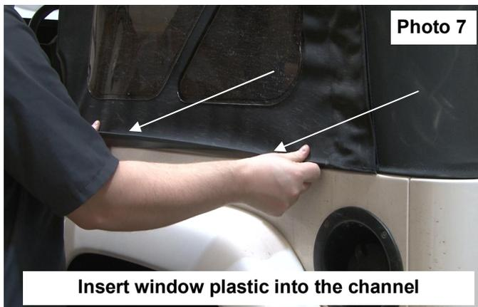
**Insert window plastic into the channel**
