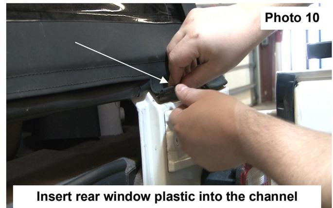
**Insert rear window plastic into the channel**
