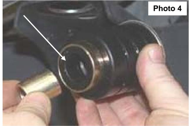
8. Install the bushings in the 3 side body locations marked **1** in the **Diagram 1**.
