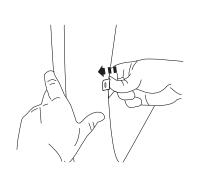
Press U-clip in place so that it encompasses both edge of fender flare and edge of fender.
