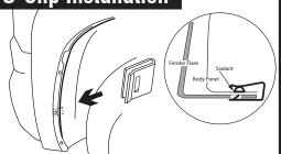
Due to building variations in trucks, it may be necessary to remove some sealant from inner lip of fender to allow installation on U-Clips.
