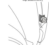
Press down on Inner Clip as indicated until an audible "snap" is heard. NOTE: This may require pliers.
