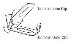
Install Protective Tab over location indicated and install Dacromet Clip Assembly is indicated on top of The Tab. (See next Step for detail of clip attachment.)
