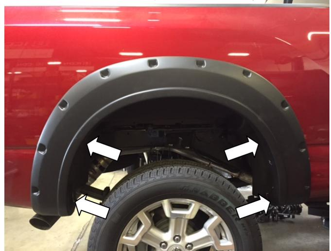
**STEP 10:** Place Fender Flare on the vehicle into the position of best fit. Note where (4) slots in Fender Flare correspond with (4) existing screws in the vehicle wheel arch molding. Remove Fender Flare. Remove only the existing vehicle screws in location as shown with a #2 Phillips head screwdriver. Maintain screws for re-install.
