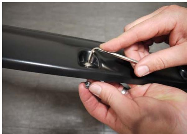
**STEP 1:** Attach the provided bolts and nuts to each Fender Flare using a 3/16" Allen key and a 10mm wrench/socket (wrench /socket and Allen key not supplied). Ensure inside of Fender Flares where the rubber seal is attached is clean, using the alcohol wipes provided. Wipe away any residue with a dry clean cloth.
