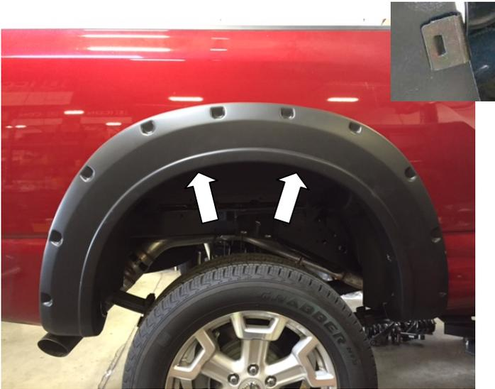
**STEP 12:** Install the provided U shape metal clips in the (2) remaining slot locations in the Fender Flare. Ensure that positive pressure is applied on the Fender Flare to the vehicle fender when installing clips. Slide the clip over the Fender Flare and the inner lip of the wheel arch ensuring that the barb in the clip locates in the slot of the Fender Flare. Ensure all fixing points are tight and secure and that the rubber seal is flush neatly against the vehicle body.
