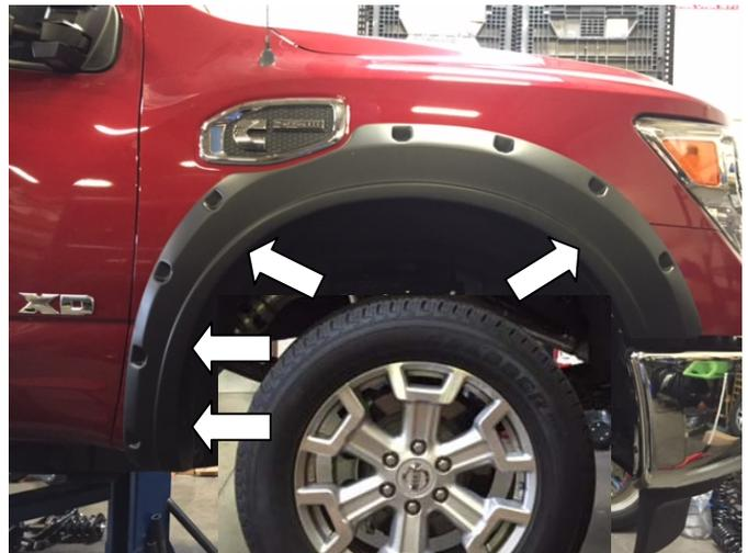
**STEP 6:** Place Fender Flare on vehicle, ensure the slots in the Fender Flare align with the holes in the wheel arch from the previously removed factory screws. Using #2 Phillips head screwdriver, re-install the previously removed (4) screws through slots in Fender Flare. Once positioned correctly ensure all fixing points are tight and secure.
