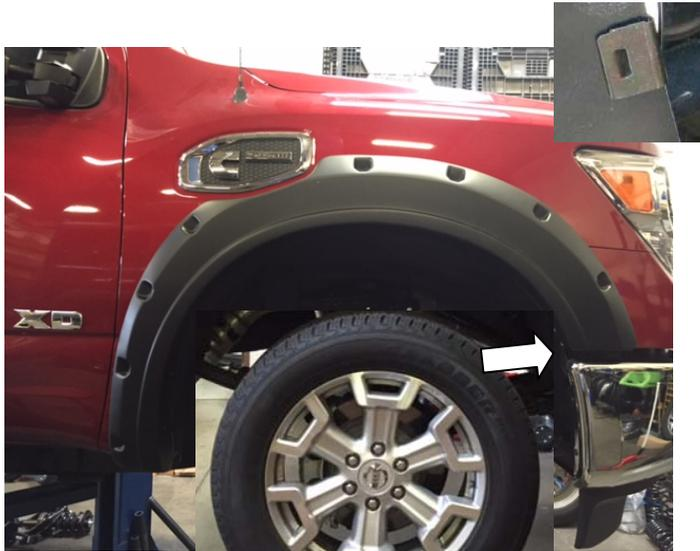
**STEP 7:** Install the provided U shape metal clip at the (1) remaining slot location in the Fender Flare. Ensure that positive pressure is applied on the Fender Flare to the vehicle fender when installing clips. Slide the clip over the Fender Flare and the inner lip of the front bumper fascia ensuring that the barb in the clip locates in the slot of the Fender Flare. Ensure that the rubber seal is flush neatly against the vehicle body.
