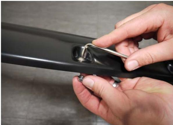
**STEP 1:** Attach the 10 bolts and nuts to each Fender Flare using a 3/16" Allen key and a 10mm wrench/socket (wrench /socket and Allen key not supplied). Ensure inside of Fender Flares where the rubber seal is attached is clean, using the alcohol wipes provided. Wipe away any residue with a dry clean cloth.
