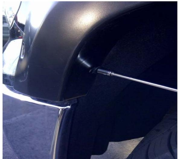
**STEP 10:** Loosely re-install factory screw through the remaining slot in the front upper wheel arch molding. Ensure Fender Flare is centered and in position of best fit on fender. Tighten all front fender fixing points to ensure a tight and secure fit and that the rubber seal is flush neatly against the vehicle body.
