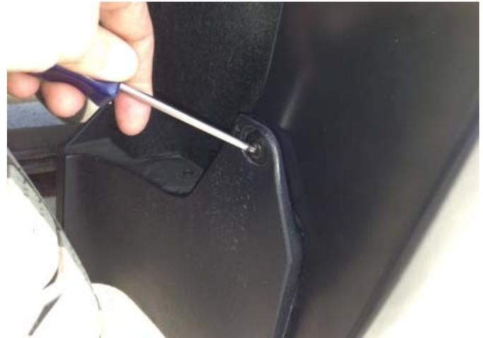
**STEP 14:** Place Fender Flare on the vehicle into the position of best fit, slide the bottom front end of Fender Flare between the existing mud flap deflector and wheel arch molding so that the slot in the Fender Flare is under the vacant hole in the mud flap. Using #15 Torx head screwdriver, loosely re-install the previously removed screw. Ensure the installed rubber seal is resting firmly on the mud flap deflector.
