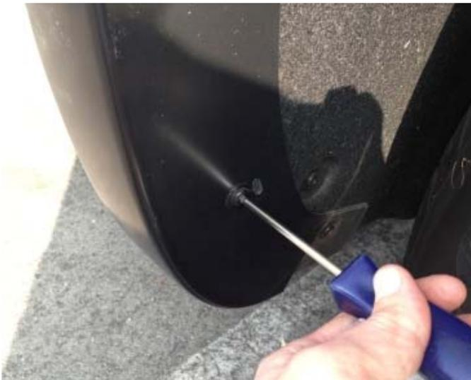
**STEP 9:** Loosely re-install previously removed factory screw through the slot in the Fender Flare at the bottom rear wheel arch molding using #15 Torx head screwdriver.
