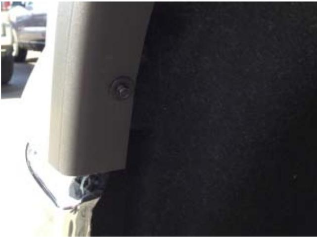
**STEP 7:** Using a 7mm or 8 mm socket, remove upper front wheel arch molding screw. Maintain screws for re-install.
