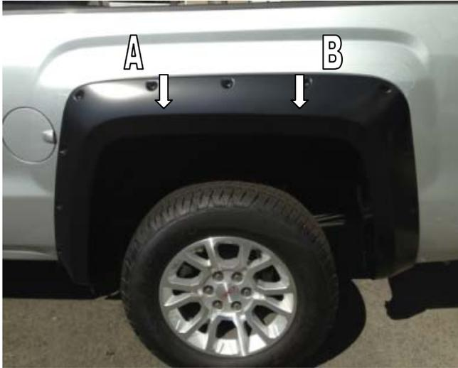
**STEP 15:** To secure the Fender Flare to vehicle body, ensure Fender Flare is in position of best fit and the slots in position **A** and **B** (Step: 11) are over the vacant holes in the wheel arch molding. Apply pressure on Fender Flare towards the vehicle fender when re-installing the previously removed factory screws in position **A** and **B** using a #15 Torx head screwdriver.
