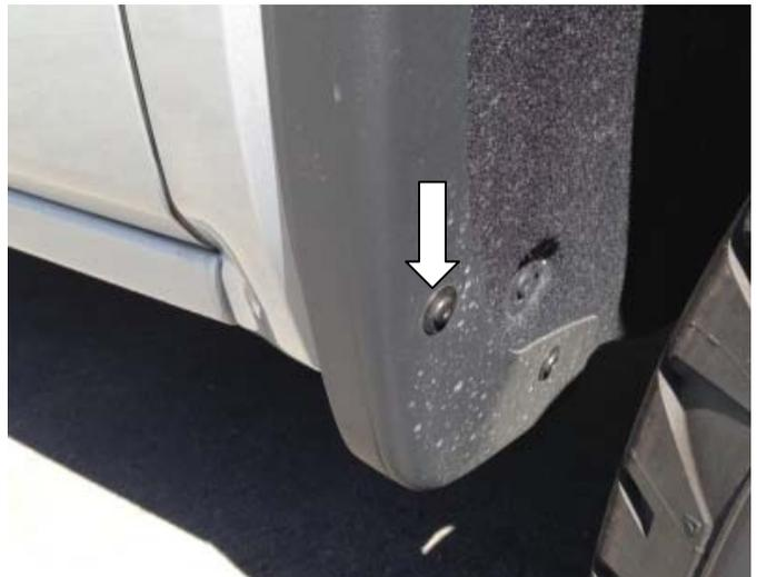
**STEP 6:** Using #15 Torx head screwdriver remove bottom rear wheel arch molding screw. Maintain screws for re-install.
