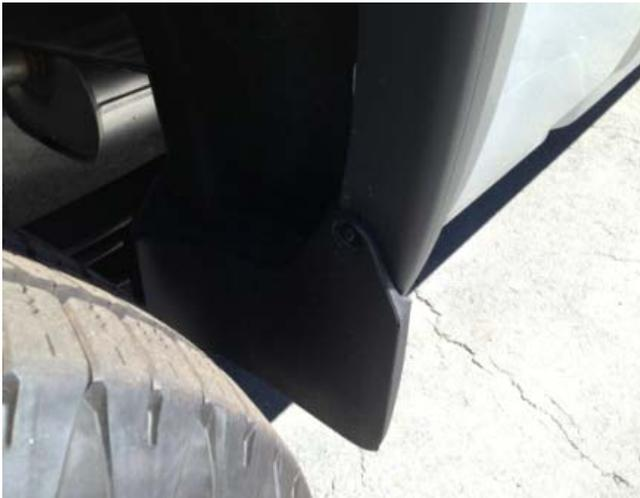
**STEP 13:** Using #15 Torx head screwdriver, remove upper screw as previously noted in position **C** from the factory mud flap deflector. Maintain screws for re-install.
