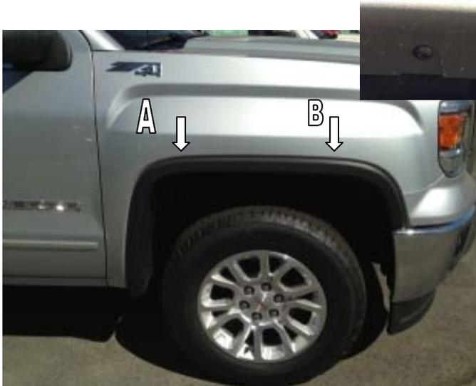
**STEP 5:** Place Fender Flare on the vehicle into the position of best fit. Note where (4) slots in Fender Flare correspond with (4) existing screws in the vehicle wheel arch molding. Remove Fender Flare. Remove the existing vehicle screws in location **A** and **B** using #15 Torx head screwdriver. Maintain screws for re-install.
