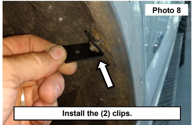
9. Install the (2) 6mm clips with the threaded side to the top on the brackets. **See Photo 9.**
