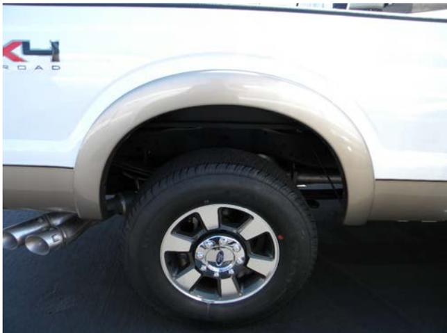
**STEP 11:** Clean the body areas where the Fender Flares will make contact. Use the supplied alcohol wipe.
