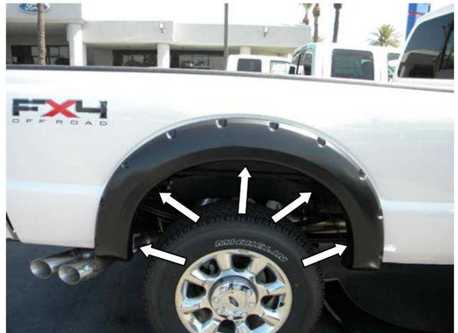
**STEP 12:** Place the Fender Flare onto the vehicle and fit into the correct position following the contours of the body. Use ten (10) of the .6mm clips (five 5 per side) to secure the Fender Flare to the body. Make sure the dimple in the clip securely attaches in the slot on the Fender Flare.
