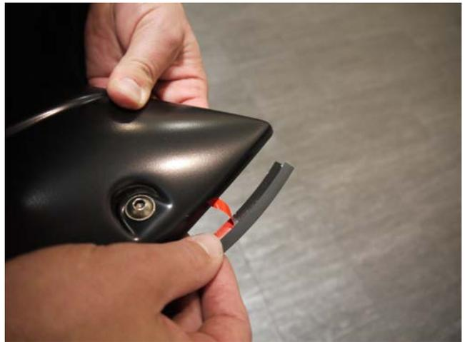
**STEP 10:** Attach the included rubber seal to the Fender Flares. Peel back 2" of the adhesive backing and position on the Fender Flare. Attach the seal to the Fender Flare, peeling back a few inches at a time. Attach rubber seal along all areas the Fender Flare will make contact with the vehicle body.
