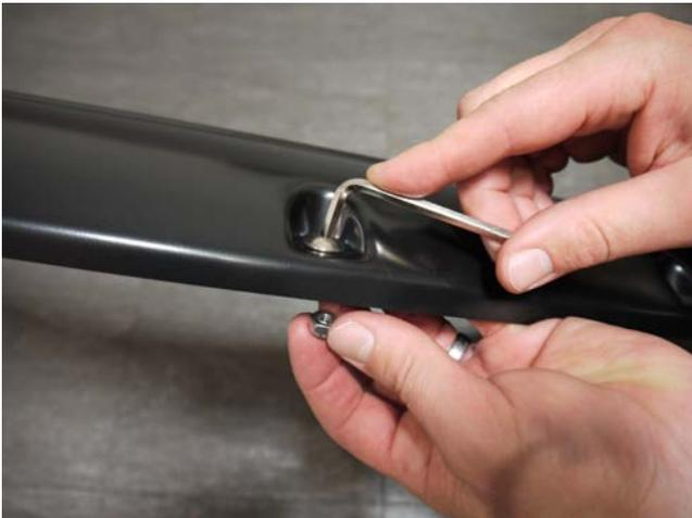
**STEP 9:** Attach 10 bolts to each Fender Flare using a 3/16" Allen key and a 10.0mm wrench/socket. (wrench/socket and Allen key not supplied). Ensure inside of Fender Flares where the rubber seal is attached is clean, using the alcohol wipes provided. Wipe away any residue with a dry clean cloth.
