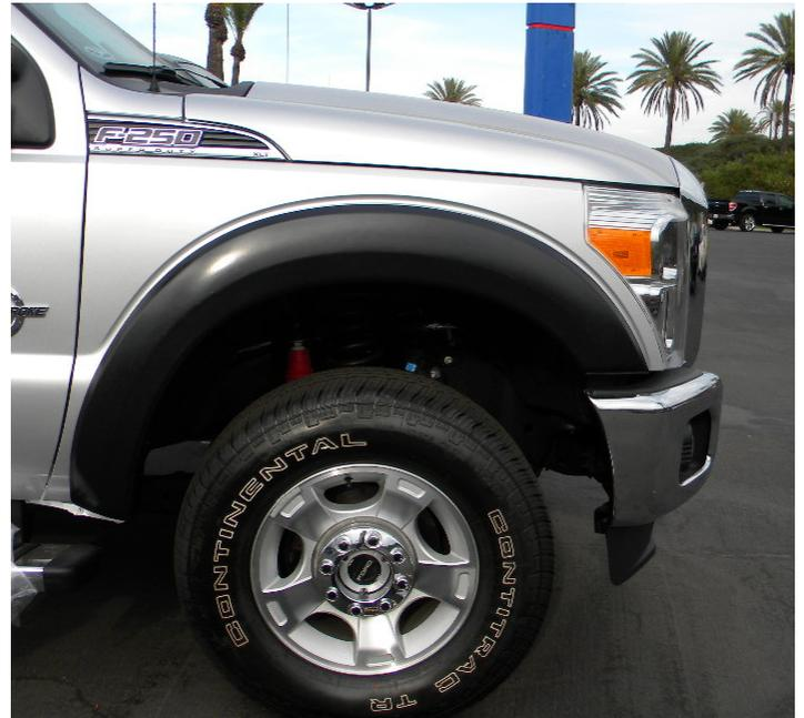
**STEP 7:** Place the Fender Flare onto the vehicle and fit into the correct position following the contours of the body. Ensure the slots in the part align with the holes in the fender from the previously removed 5.5mm socket head screws.
