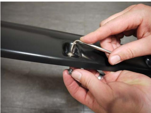
**STEP 1:** Attach 9 bolts to each Fender Flare using a 3/16" Allen key and a 10.0mm wrench/socket. (wrench/socket and Allen key not supplied). Ensure inside of Fender Flares where the rubber seal is attached is clean, using the alcohol wipes provided. Wipe away any residue with a dry clean cloth. For model year 2011 and newer, only 8 bolts are use.
