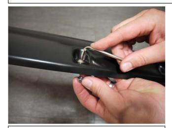
**STEP 1:** Attach 9 bolts to each Fender Flare using a 3/16" Allen key and a 10.0mm wrench/socket. (wrench/socket and Allen key not supplied). Ensure inside of Fender Flares where the rubber seal is attached is clean, using the alcohol wipes provided. Wipe away any residue with a dry clean cloth.
