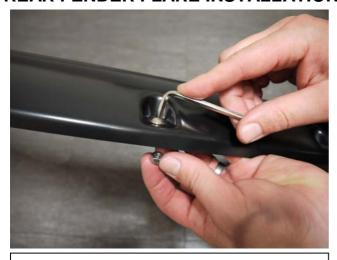
**STEP 9:** Attach 10 bolts to each Fender Flare using a 3/16" Allen key and a 10.0mm wrench/socket. (wrench/socket and Allen key not supplied). Ensure inside of Fender Flares where the rubber seal is attached is clean, using the alcohol wipes provided. Wipe away any residue with a dry clean cloth.
