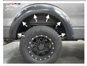
**STEP 12:** Place the Fender Flare onto the vehicle and fit into the correct position following the contours of the body. Use twelve (12) of the .6mm clips (six (6) per side) to secure the Fender Flare to the body. Make sure the dimple in the clip securely attaches in the slot on the Fender Flare.
