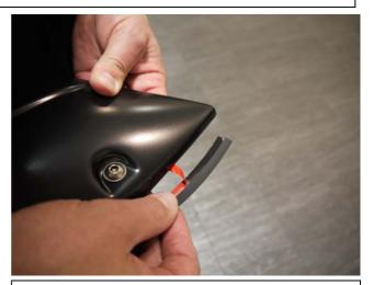
**STEP 2:** Attach the included rubber seal to the Fender Flares. Peel back 2" of the adhesive backing and position on the Fender Flare. Attach the seal to the Fender Flare, peeling back a few inches at a time. Attach rubber seal along all areas the Fender Flare will make contact with the vehicle body.
