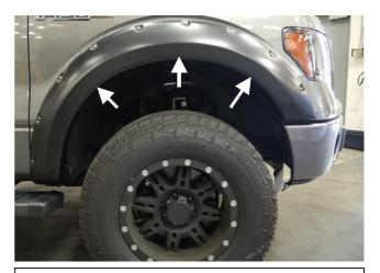
**STEP 8:** Insert six (6) of the .9mm lever retaining clips (three (3) per side) into the Fender Flare. Make sure the tab in the clip securely attaches in the slot on the Fender Flare. Secure with four (4) bolts removed in Step 6. For 2007-2013 vehicles, secure the center clip with the included scrivet.
