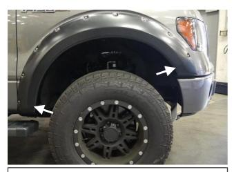
**STEP 7:** Place the Fender Flare onto the vehicle and fit into the correct position following the contours of the body. Use four (4) of the .6mm clips (two (2) per side) to secure the Fender Flare to the body. Make sure the dimple in the clip securely attaches in the slot on the Fender Flare.
