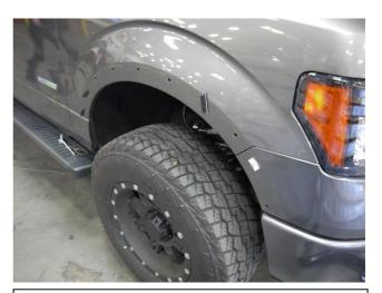
**STEP 6:** Remove four (4) 5.5mm bolts and retain for installation of Fender Flares. For 2007-2013 vehicles, only 3 bolts are removed.
