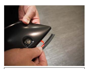
**STEP 10:** Attach the included rubber seal to the Fender Flares. Peel back 2" of the adhesive backing and position on the Fender Flare. Attach the seal to the Fender Flare, peeling back a few inches at a time. Attach rubber seal along all areas the Fender Flare will make contact with the vehicle body. Trim any excess rubber seal
