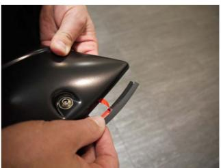
**STEP 13:** Attach the included rubber seal to the Fender Flares. Peel back 2" of the adhesive backing and position on the Fender Flare. Attach the seal to the fender flare, peeling back a few inches at a time. Attach rubber seal along all areas the Fender Flare will make contact with the vehicle body. Trim any excess rubber seal.
