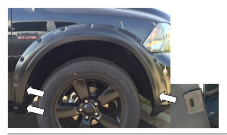
**STEP 11:** Re-install the x2 previously removed screws from STEP 7 using 8.0mm socket. To secure the front slot in the Fender Flare to the body, take the black metal clip and slide it over the Fender Flare and the front bumper lip. Position the clip so that the barb in the clip locates in the slot of the Fender Flare. Ensure all fixing points are tight and secure and that the rubber seal is flush neatly against the vehicle body.
