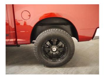
**STEP 14:** Clean the body areas where the Fender Flares will makes contact.. For models equipped with factory fender flares, removal of factory flares is required, please consult the vehicle service manual for factory fender flare removal.
