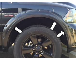
**STEP 10:** Check fitment and contour of Fender Flare to headlight housing and readjust if necessary. Re-install all bolts removed in step 9 using 8.0mm socket.
