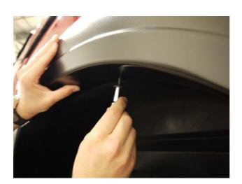
**STEP 16:** Re-install all bolts removed in step 14 using 8.0mm socket.
