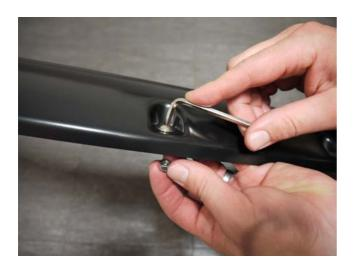
**STEP 12:** Attach 11 bolts to each Fender Flare using a 3/16" Allen key and a 10.0mm wrench/socket. (wrench/socket and Allen key not supplied) Ensure inside of Fender Flares where the rubber seal is attached is clean, using the alcohol wipes provided. Wipe away any residue with a dry clean cloth.
