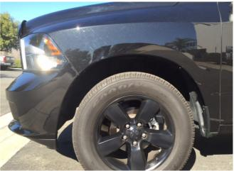
**STEP 6:** Clean the body areas where the Fender Flares will make contact. For models equipped with factory fender flares, removal of factory flares is required, please consult the vehicle service manual for factory fender flare removal.
