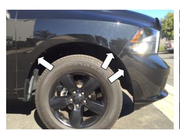
**STEP 9:** Remove all factory bolts that align with slots in part as shown using 8.0mm socket, retain screws for installation of Fender Flares.
