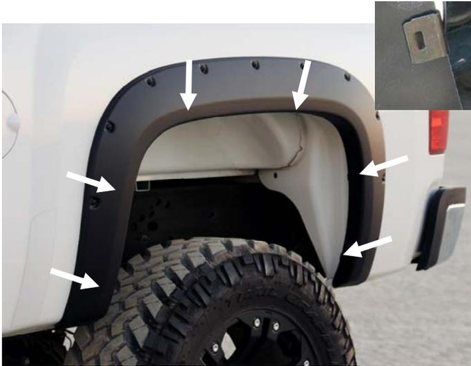
**STEP 11:** To secure the Fender Flare to the body, take the black metal clips and slide them over the Fender Flare and the inner wheel arch lip. Position the clip so that the barb in the clip locates in the slot of the Fender Flare. Ensure all fixing points are secure and that the rubber seal is flush neatly against the body.
