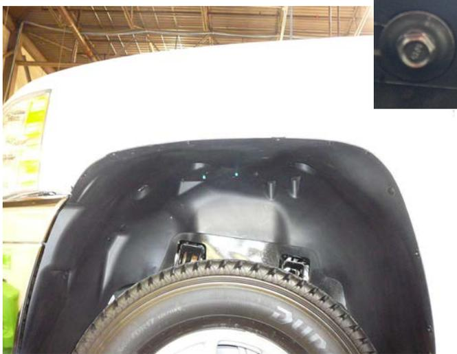
**STEP 5:** Place the Fender Flare on the vehicle into the position of best fit. Note where the slots in Fender Flare align with the existing screws in the vehicle. Remove Fender Flare. Use the original manufacturer's hardware that is in the wheel arch of the vehicle to fit the Fender flares. Remove the x6 9/32" (7mm) socket head screws from the fasteners on the vehicle.
