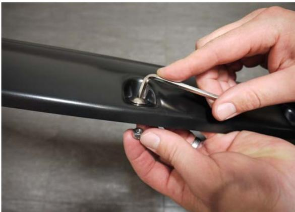
**STEP 1:** Attach the 9 bolts, washers and nuts to each Fender Flare using a 3/16" Allen key and a 10.0mm wrench/socket. (wrench/socket and Allen key not supplied). Ensure inside of Fender Flares where the rubber seal is attached is clean, using the alcohol wipes provided. Wipe away any residue with a dry clean cloth.
