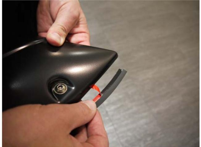
**STEP 8:** Attach the included rubber seal to the Fender Flares. Peel back 2" of the adhesive backing and position on the Fender Flare. Attach the seal to the Fender Flare, peeling back a few inches at a time. Ensure pressure is used to secure rubber seal to Fender Flare edge. Attach rubber seal along all areas the Fender Flare will make contact with the vehicle body.
