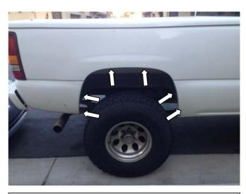
**STEP 13:** Install the supplied screw plugs into the existing holes in wheel arch as show.
