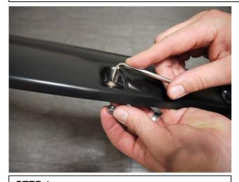
**STEP 1:** Attach supplied bolts and nuts to each Fender Flare using a 3/16" Allen key and a 10.0mm socket. (wrench/socket and Allen key not supplied) Ensure inside of Fender Flares where the rubber seal is attached is clean, using the alcohol wipes provided. Wipe away any residue with a dry clean cloth.
