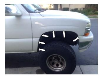
**STEP 6:** Install the supplied screw plugs into the existing holes in wheel arch as show.
