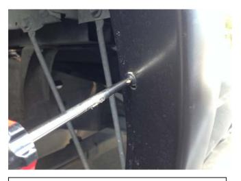
**STEP 7:** Place the Fender Flare onto the vehicle and fit into the correct position following the contours of the body. Locate the mounting slots in the part over the installed screw plugs. Install screws through the screw plugs as shown. Repeat installation method for other side. Double check the front Fender Flares to make sure all screws are tight securely fastened.
