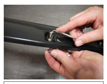
**STEP 8:** Attach supplied bolts and nuts to each Fender Flare using a 3/16" Allen key and a 10.0mm. (wrench/socket and Allen key not supplied) Ensure inside of Fender Flares where the rubber seal is attached is clean, using the alcohol wipes provided. Wipe away any residue with a dry clean cloth.
