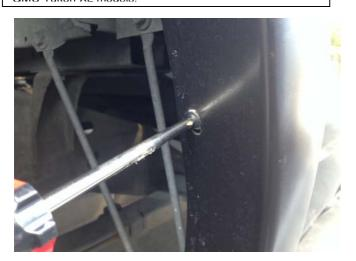
**STEP 14:** Place the Fender Flare onto the vehicle and fit into the correct position following the contours of the body. Locate the mounting slots in the part over the installed screw plugs. Install screws through the screw plugs as shown. Repeat installation method for other side. Double check the rear Fender Flares to make sure all screws are tight securely fastened.
