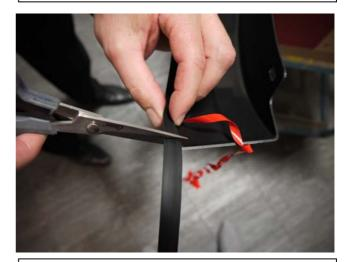
**STEP 11:** Trim any unnecessary extrusion and discard.
