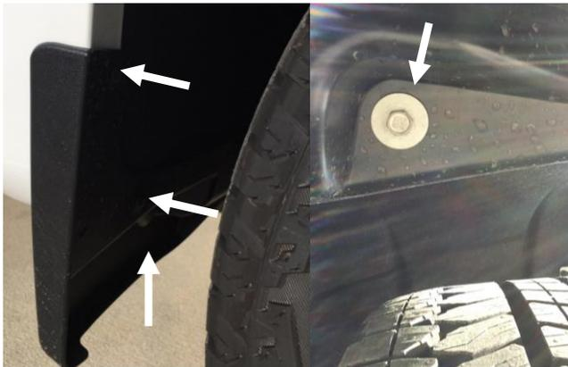
**STEP 5:** For models **WITH FRONT** factory mud guards, remove using #15 Torx head screwdriver at the upper and lower screw locations from the front factory mudguards and M10 socket at the underside location indicated above, maintain #15 Torx head screws for re-install. Retain factory mudguards for later use if required, Fender Flares require the mud guards to be removed.
