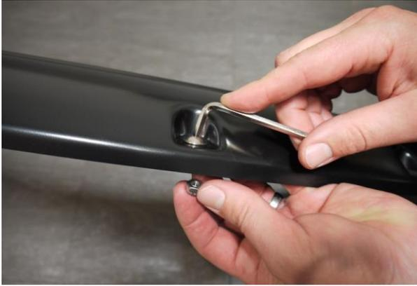
**STEP 10:** Attach the bolts and nuts to each Fender Flare using 3/16" Allen Key/Torx and a 1/2" wrench/socket (wrench/socket and Allen key not supplied). Ensure inside of Fender Flares where the rubber extrusion is attached is clean, using the alcohol wipes provided. Wipe away any residue with a dry clean cloth.
