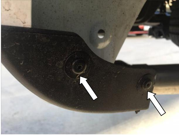
**STEP 14:** Using #15 Torx head screwdriver remove the two bottom screws from the rear factory mud guard. Maintain screws for re-install.
