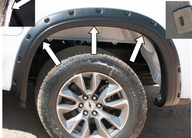
**STEP 17:** To secure the Fender Flare to the body, apply upward tension on Fender Flare to the vehicle fender when installing the black metal clips. Slide the clips over the Fender Flare and the inner wheel arch lip in the three locations shown. Position the clip so that the barb in the clip locates in the slot of the Fender Flare. Ensure all mounting points are tight and secure and that the extrusion is flush neatly against the vehicle body. Repeat install steps for the opposite side.
