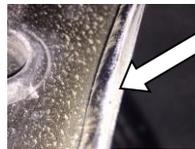
**Note:** Inner sealant bead in wheel well.
