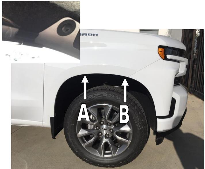
**STEP 6:** Place Fender Flare on the vehicle into the position of best fit. Note where the slots in Fender Flare at positions **A, B** and vehicle wheel arch. Remove Fender Flare. Place the small abrasive resistant tapes over the fender lip at the noted positions **A, B**. Slide the large clips over the inner fender panel at the noted **A, B** positions, ensure the hook on the back of the clip engages over the fender lip.
