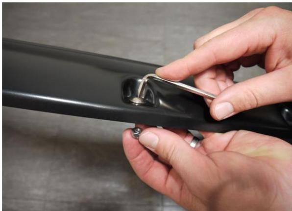
**STEP 1:** Attach the bolts and nuts to each Fender Flare using a 3/16" Allen key/Torx and a 1/2" wrench/socket. (wrench /socket and Allen key not supplied). Ensure inside of Fender Flares where the rubber extrusion is attached is clean, using the alcohol wipes provided. Wipe away any residue with a dry clean cloth.
