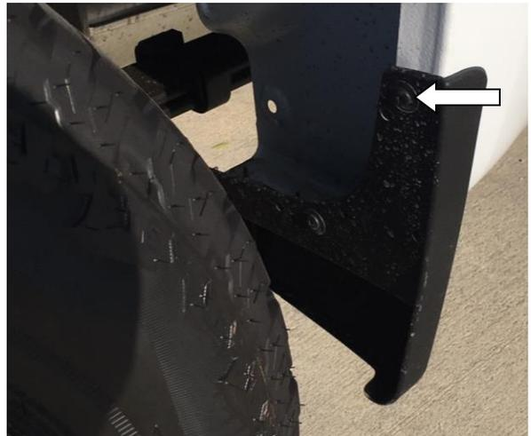
**STEP 13:** Using #15 Torx head screwdriver remove upper screw from the front factory mud guard in the rear wheel arch. Maintain screws for re-install.
