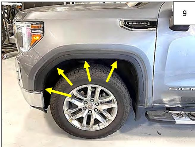
Hold flare firmly on vehicle. Using a grease pencil, mark 4 hole locations through flare onto fender lip.
