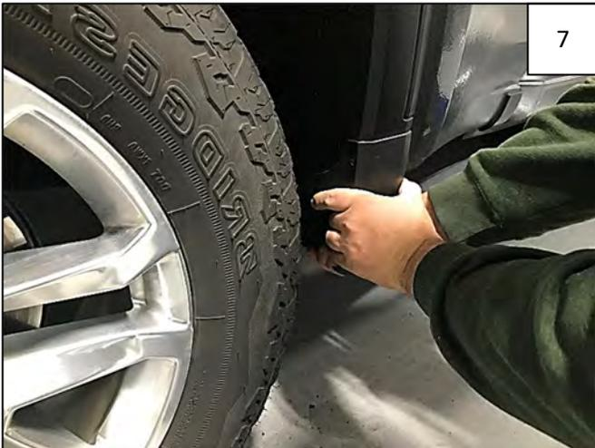
Using a quick jerking motion down and toward you, pry forward mud guard from vehicle and discard.
