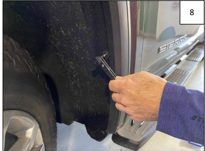
Remove 1 T-15 factory screw from wheel well (above mud guard area).
