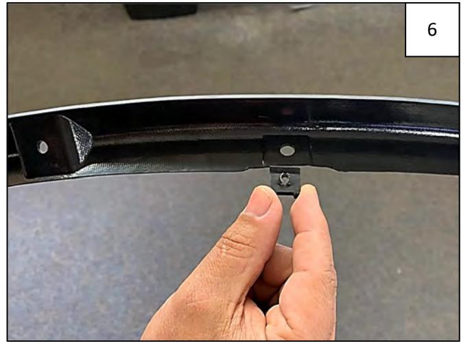
Install 3 Short "U" Clips onto the Inner Bracket as shown. NOTE: Driver's side Inner Bracket is marked with an "LH" and the passenger's side Inner Bracket is marked with an "RH".
