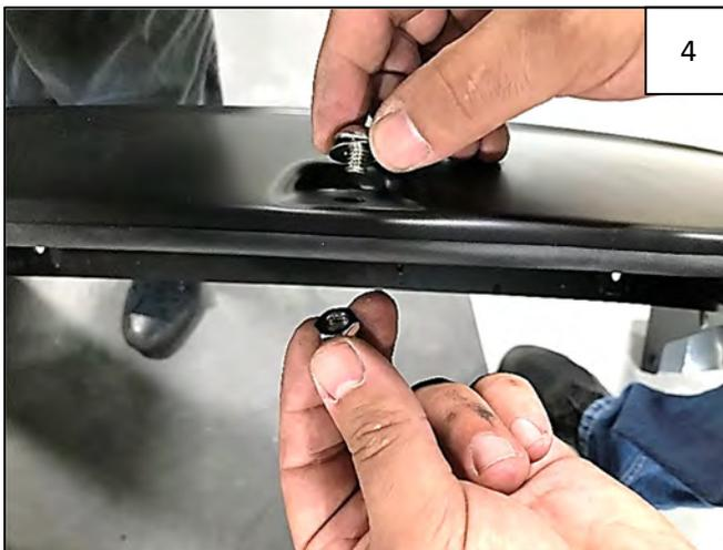
Place a supplied Pocket Nylock Nut over the end of each bolt and tighten using a 1/2" wrench for the Nut and the supplied T-45 Torx Bit for the Bolt. Repeat for all pockets.
