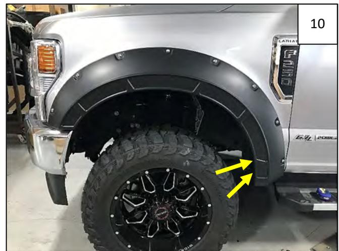
Still pressing flare to fender, reinstall 2 remaining factory screws removed in Step 5. Apply pressure to flare towards vehicle body at each fastening point and tighten all fasteners.
