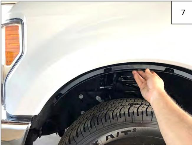
Line up holes in the Inner Bracket with the 4 upper-most factory holes in wheel well.
