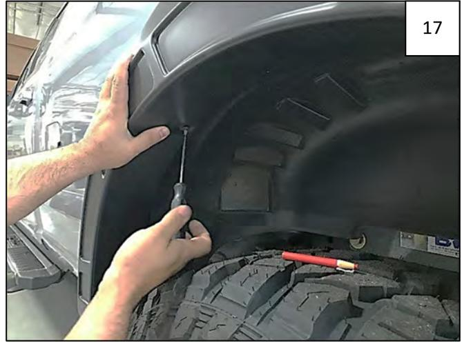
While holding flare to vehicle, start supplied Truss-Head Screws through the 4 topmost mounting holes in flare and into clips installed in Step 16. Apply pressure to flare towards vehicle body at each fastening point and tighten all fasteners.
