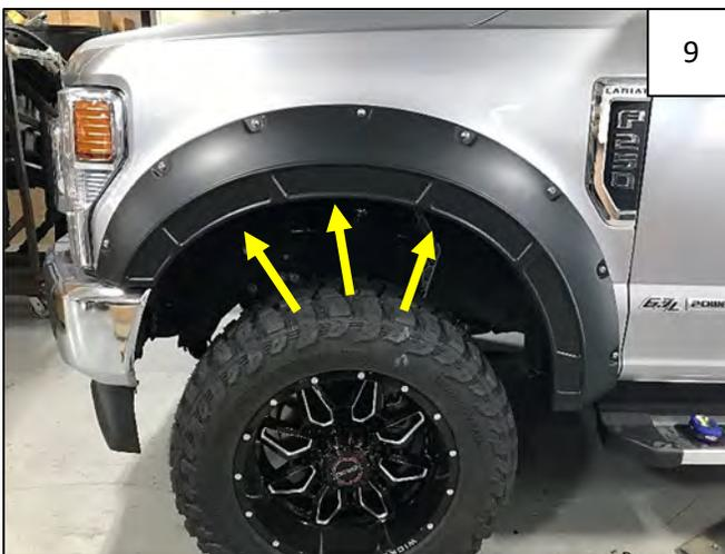
Aligning flare on fender, press inward on the flare to line up the flare mounting holes with the clips on the Inner Bracket. Install 3 supplied Truss-Head Screws through the flare and into the inner piece. Do not tighten.
