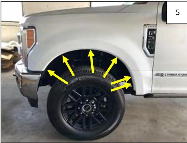
Remove 6 factory screws with a 7/32" socket wrench. Retain screws for reinstallation. NOTE: For Platinum Edition, there are additional screws to be removed and retained.
