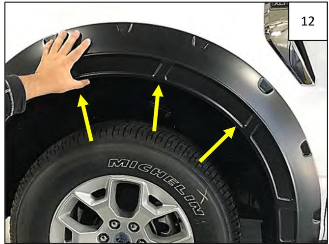
Aligning flare on fender, press inward, firmly with force, on the flare to line up the flare mounting holes with the clips on the Inner Bracket. Install 3 supplied Truss-Head Screws through the flare and into the Inner Bracket. Do not tighten.
