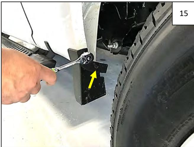
Using a 7mm socket, remove 2 factory screws from lower front of wheel well. Retain screws.
