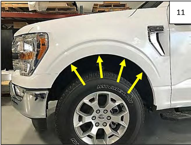
Using a 7mm socket, reinstall 4 factory screws through the Inner Bracket and into fender. Tighten these screws.
