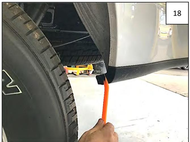
Using a pry tool, remove outer factory plastic fastener from lower rear of wheel well. Discard. Leave inner plastic fastener installed.
