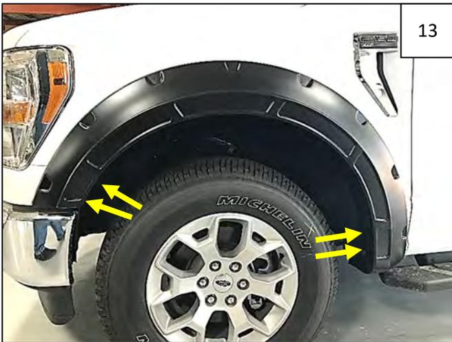
Still pressing flare firmly to fender, reinstall 4 remaining factory screws removed in Step 5. Apply pressure to flare towards vehicle body at each fastening point and tighten all fasteners.
