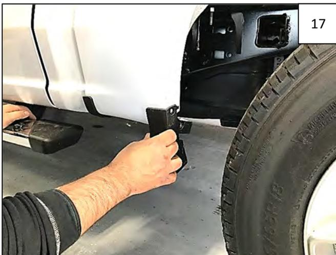
Remove and discard plastic trim by pulling firmly away from vehicle, disengaging a hidden factory clip inside.
