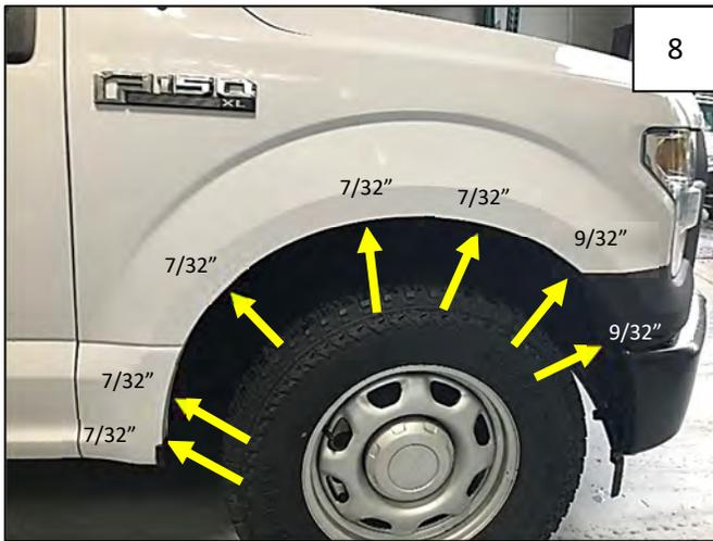
Remove 5 factory screws with a 7/32" Socket. Remove 2 front-most factory screws with 9/32" Socket. Retain Screws for reinstallation. **NOTE:** For Platinum Edition, additional screws will need to be removed and saved for reinstallation.
