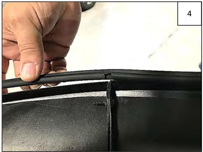
When you come to the jointure of the flare and extension piece, cut a notch in the back of the edge trim.
