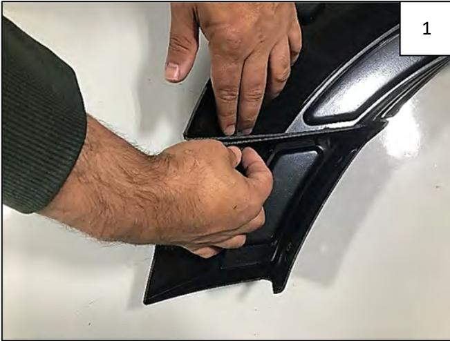
Install Extension Pieces to main front flares using 2 supplied #8 Speed Clips and #8 Screws per side.
