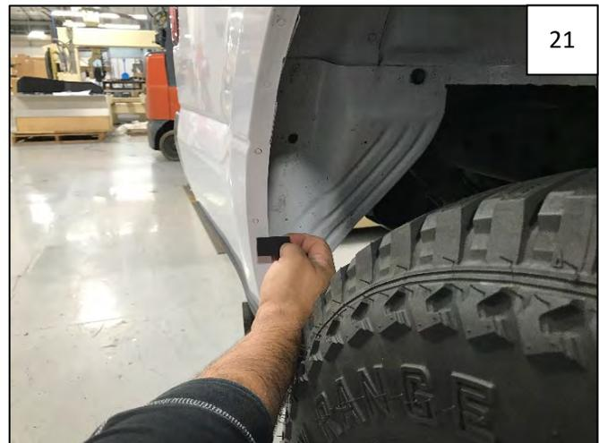
Peel liner from a supplied Foam Tab and wrap around wheel well sheet metal, centering over each mark made in Step 19 (four places).
