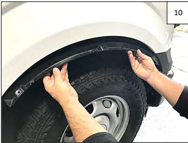
Line up the holes in the Inner Bracket with the 3 uppermost factory holes, installing correct Inner Bracket for each side.
