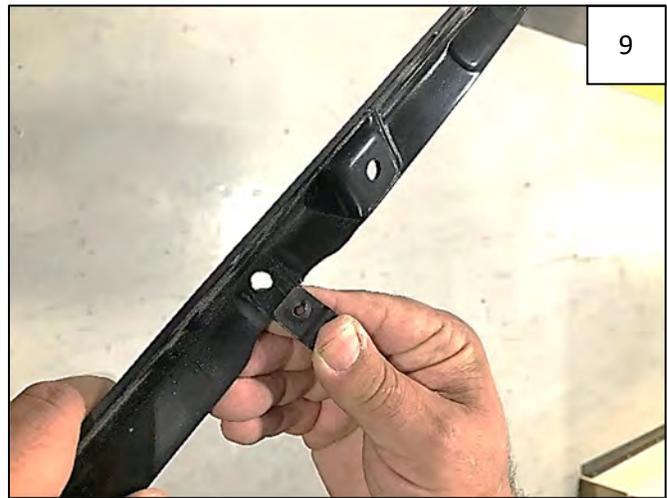
Attach 3 #10 "U" Clips to each Inner Bracket over pre-drilled holes as shown. **NOTE:** Driver Side Inner Bracket is marked with an "LF" and Passenger Side Inner Bracket is marked with an "RR."
