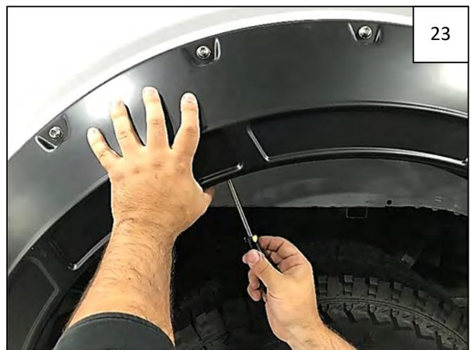
While holding flare to vehicle, start supplied #10 Truss Screws through the 4 topmost mounting holes in flare and into clips installed in Step 22.
