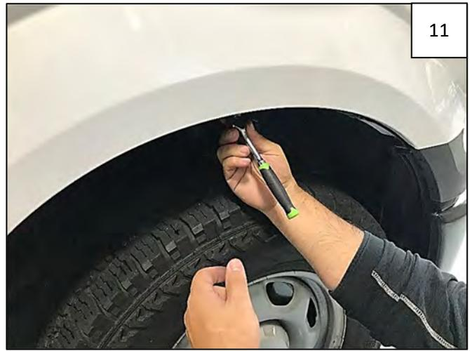
Using a 7/32" Socket, reinstall 3 top factory screws through the holes in the Inner Bracket. Tighten screws.
