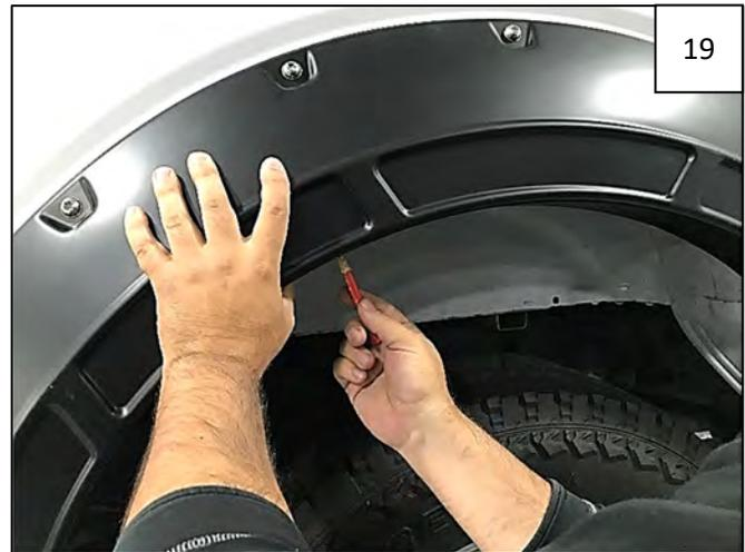
Hold flare to vehicle and mark 4 flare hole locations with a grease pencil.
