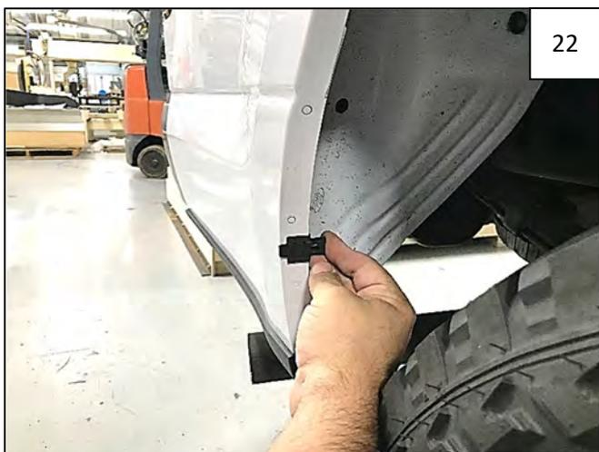
Install a supplied Long "U" Clip over each Foam Tab.
