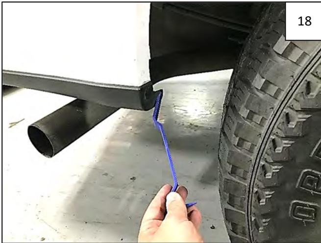
Using a pry tool, remove plastic factory fastener from rear of wheel well.
