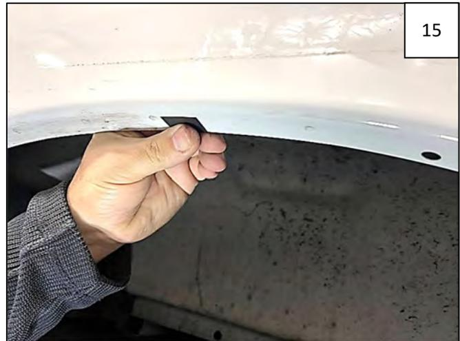
For topmost hole in wheel well, peel liner from a supplied Mounting Tab and center over the factory hole. If vehicle had full wheel well liners, no tab or clip is needed – just reuse factory fastener.
