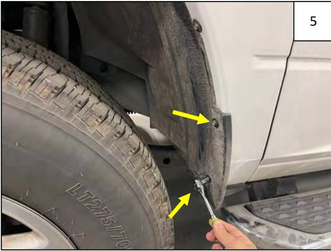
Remove 2 factory screws from mud flap. Fasteners will be reused. Do not remove fastener above mud flap. Pull mud flap towards you to remove – it's held on with 2 hidden plastic clips.
