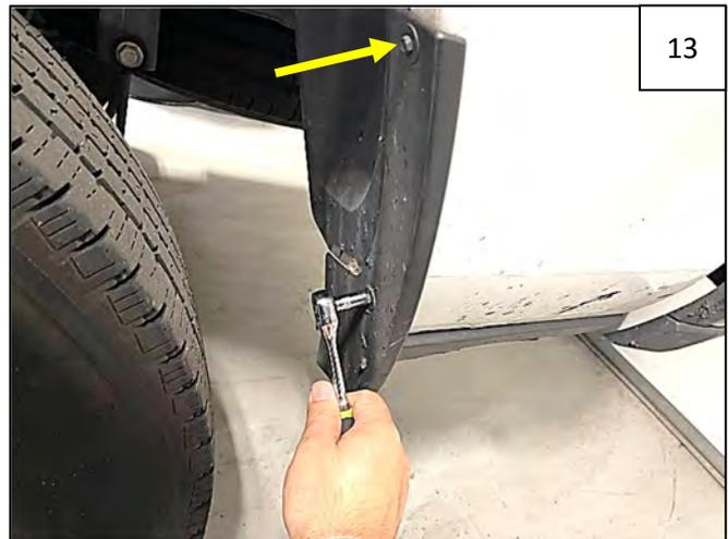
Using an 8mm socket, remove 2 fasteners at rear mudflap. Retain factory screws. Pull until plastic clips release.
