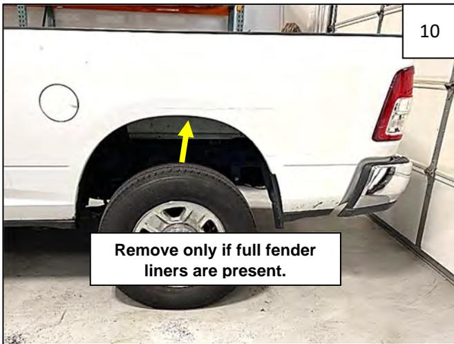
If vehicle is equipped with full fender liners, remove top most factory screw at top of fender; retain for reuse. If vehicle is not equipped with fender liners, proceed to Step 11.
