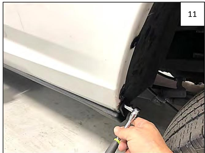
Using an 8mm socket, remove and retain factory screw at front of rear wheel well (this screw holds the underside trim on vehicle at wheel well).
