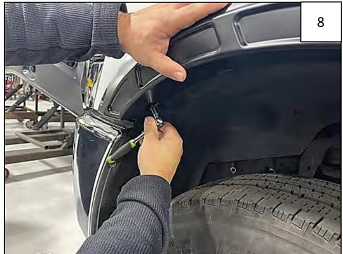
Press inward on flare to apply pressure to the flare and tighten all screws.
