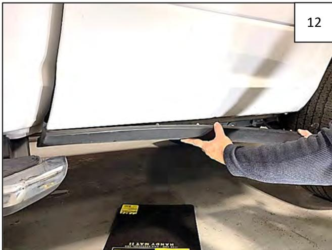
Pull underside trim off. Pull until plastic clips release. Clips may break in the process. Discard trim.
