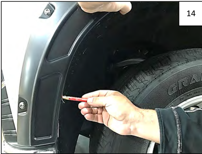
Align flare on vehicle and mark 2 forward hole locations with a grease pencil.
