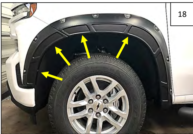
Align flare on vehicle and start 4 supplied Truss-Head Screws through holes in flare and into fender as shown.
