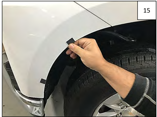
Peel liner from a supplied Foam Tab and center tab over each mark made in Step 14, folding over wheel well lip.
