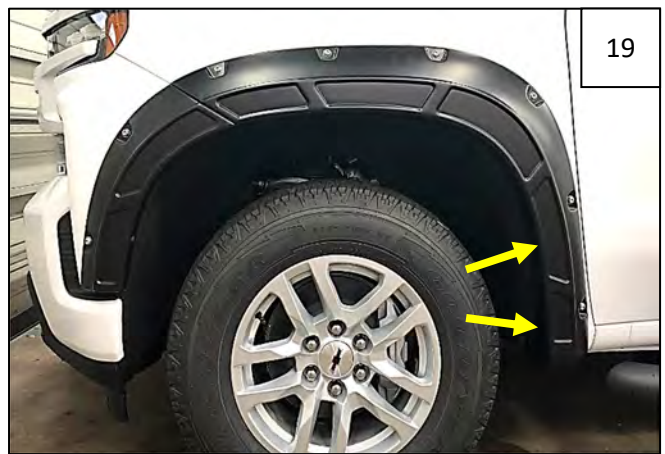
Start 2 factory T15 Torx screws at bottom rear of wheel well as shown. Apply pressure to flare towards vehicle body at each fastening point and tighten all fasteners.
