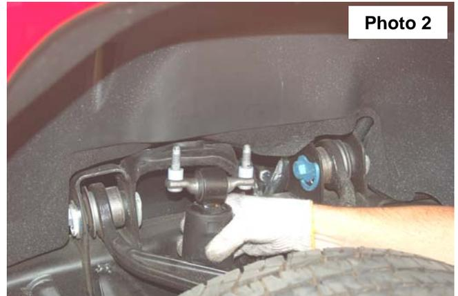
5. Measure and take note of how much thread is remaining on the torsion bar adjuster bolt. You will reset the bars at this same location with the new adjusters.
