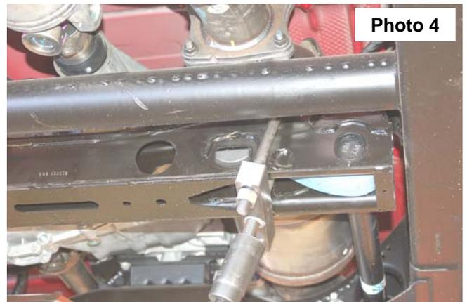
10. Install the new torsion bar adjuster just as the stock was removed.
