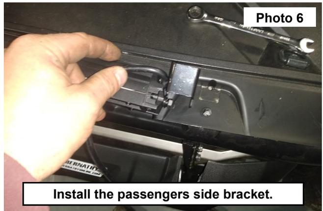
7. Place the light brackets in-between the bumper bracket and the frame mount on the Driver and Passengers side frame mount bumper bolts. **See Photos 7.**
