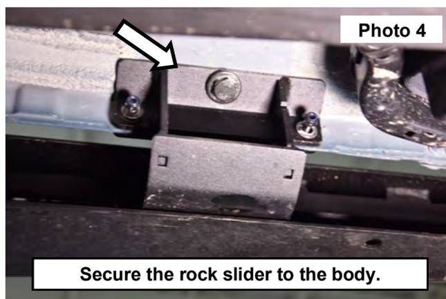
4. Place the bolt plate through the rocker into the bracket and secure using (2) of the supplied 6mm flat washers and (2) 6mm lock nuts onto the studs. Tighten using a 10mm socket. **See Photo 5.**
