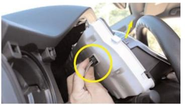
14. Connect the male end of the Speedometer Calibrator Harness to the factory wiring harness and the female end into the Instrument Panel Cluster.
