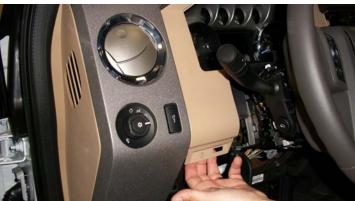
16. Return the gear selector to the Park position and turn the ignition to the OFF position. Using a 7mm socket, remove the (2) retaining screws.
