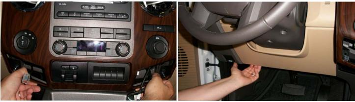
10. Remove the top and bottom of the Steering Column shroud. Using a 5.5mm socket, remove the (3) retaining screws, located below the steering column.
