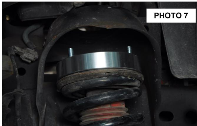
11. Reinstall the lower strut bolt using a 19mm wrench as removed in step 6.
