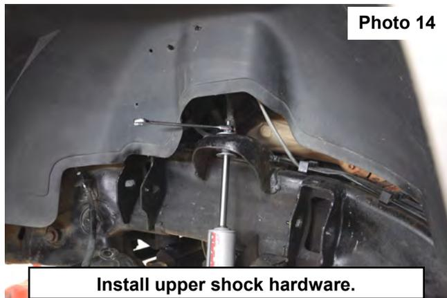
18. Tighten upper shock nut, using a 14mm wrench, until the bushings just start to bulge past the cup washers.
