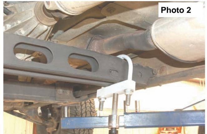
Reinstall the threaded block and adjuster bolt.
