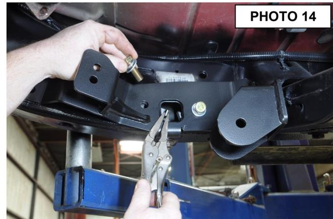
29. Install the double flag nut into the frame rail from the outside of the frame using the supplied 1/2" x 1.5" bolts, flat washers, and lock washers. Do not tighten at this time. **See Photo 15.**
