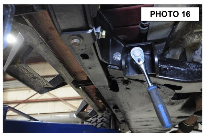
31. Torque the (4) 1/2" bolts to 65ft/lbs using a 3/4" socket. **See Photo 17.**
