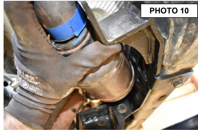
15. Once you have the correct position, tack weld the exhaust at both ends. It is recommended to double check that there is no clearance issues and then place a small bead of weld on both ends of the exhaust to ensure there is no movement during removal. **See Photos 11 & 12.**
