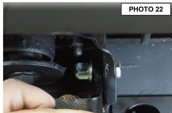
29. Install the supplied flag nuts, longer flag goes to the rear, into the frame and attach using the supplied 1/2" x 1.5" bolts and lock washers (78630BAG3). Do not tighten at this time. On the driver side bracket, you will use the flag nut that has the S shape for the bottom hole, it has to be installed first. Use the supplied 12mm x 35mm bolt and washer (78630BAG3) for the bottom hole on the passenger side bracket. **See Photo 23.**
