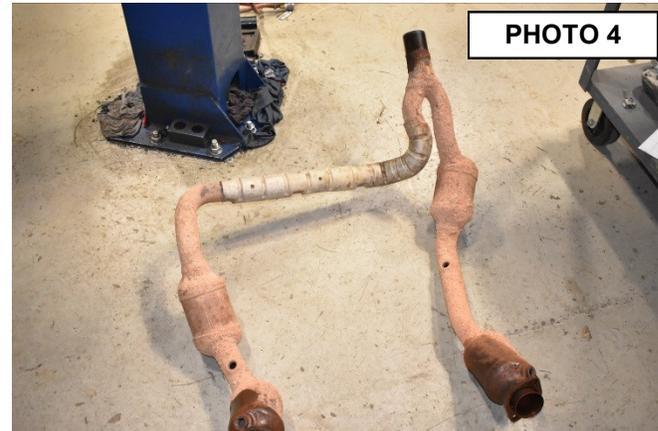
9. Clean the exhaust Y-pipe using a wire brush.
