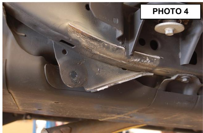
13. Place a piece of cardboard or thin sheet metal between the fuel tank and inside of the frame, this will help keep sparks off the fuel tank while cutting the inside of the lower control arm pocket.
