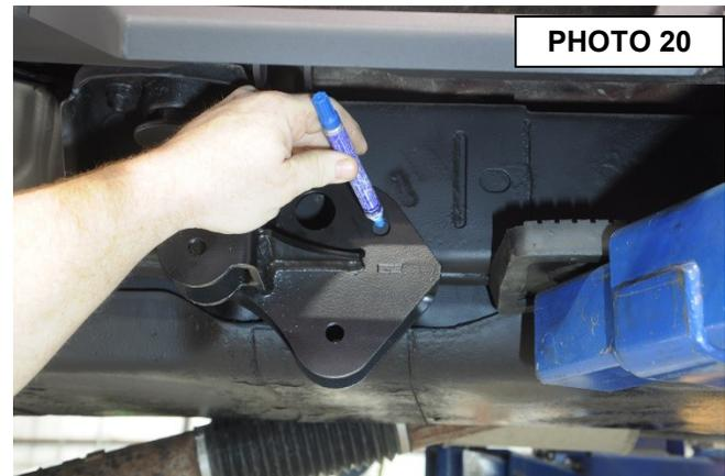
27. Drill the marked holes using a 17/32" drill, **only through the outside wall of the frame rail.** (Passenger side will have 2 17/32" holes in the frame and 1 17/32" hole in the body mount. Driver side will have 3 17/32" holes in the frame rail, 1 1-1/4" hole in the frame rail and 1 17/32" hole in the body mount.) **See Photo 21.**
