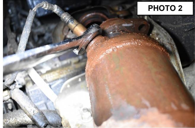
7. Using a 16mm wrench to loosen the exhaust clamp at the rear of the Y-pipe. **See Photo 3.**
