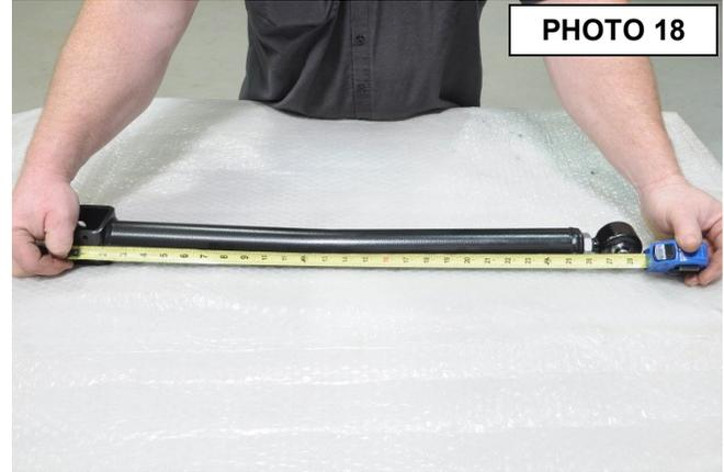
34. Install the larger supplied flex joints in the supplied front lower control arms and adjust to a length of 33.5" center to center. **See Photo 19.**
