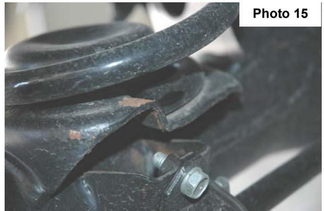
9. Using a 12mm wrench, reinstall the brake line bracket on the drivers side, and ABS bracket on the passengers side.
