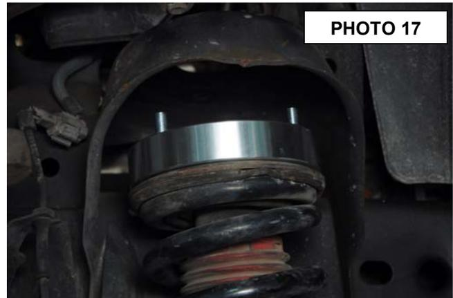
20. Position the strut assembly to reinstall the lower strut bolt in its original position that it was removed. Using original hardware and a 19mm socket torque to 100ft lbs.
