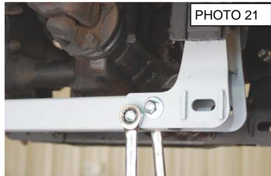
24. Install the factory cross-member section removed in step 13 with the factory hardware using a 17mm wrench. Also install the factory hardware on the differential mount using a 15mm wrench. **See Photo 22.** A straight edge must be used on the bottom of the two new brackets and the factory center bracket to assure the brackets are straight. Tighten the 4 factory center cross-member bolts. The cross-member must be straight to allow the vehicle to be re-aligned.
