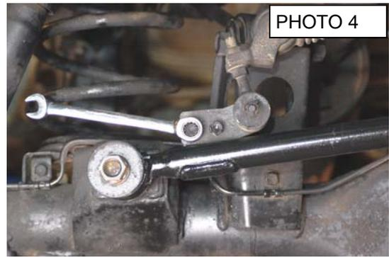
9. Remove the track bar from the axle and the frame using a 22mm wrench. **See Photo 5.**
