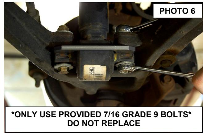
9. Retighten upper strut bolts to correct torque spec with 18mm wrench. Install the wheels / tires, using a 21mm deep well socket. Repeat steps 3-9 on Driver Side.
