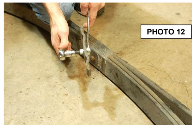
19. Using a die-grinder or air chisel remove the three factory rivets on the hanger bracket. **See Photo 13.**
