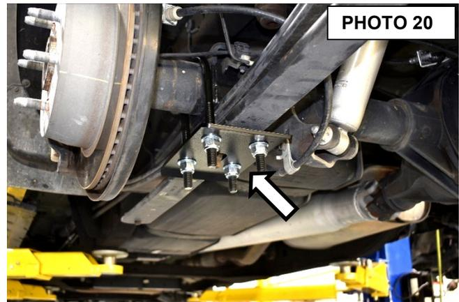
29. Using a 22 mm socket, tighten the u-bolt nuts. Torque to 90ft-lbs using an X pattern. **See Photo 21**
