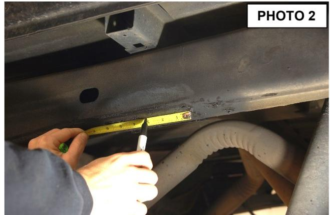
5. Drill a 11/32” hole and install the stock bolt along with the factory bump stop.
