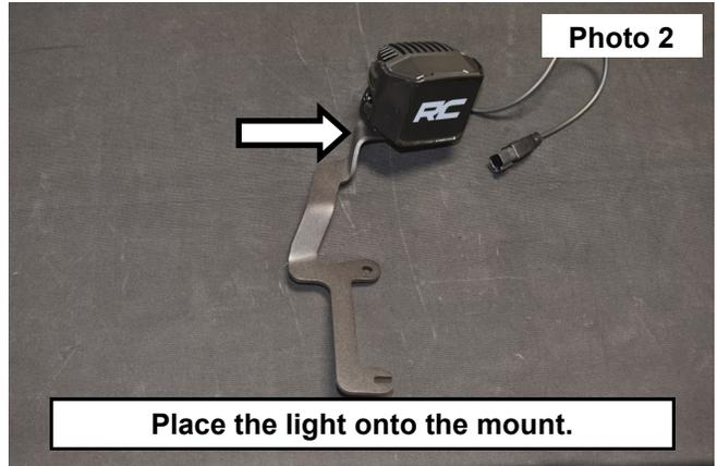
3. Secure using the supplied hardware in the light kit. Snug the light to the bracket using a 13mm wrench. **See Photo 3.**
