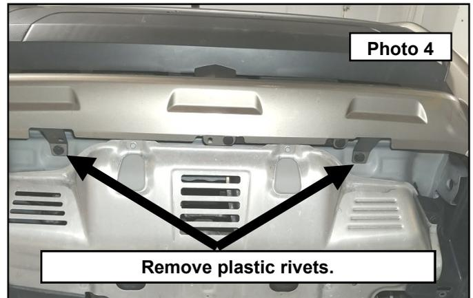
7. Under the hood, locate and remove the plastic rivets. **Photo 5**
