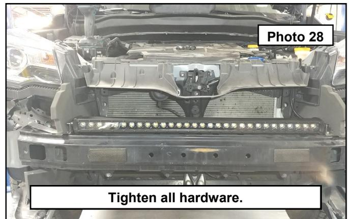
7. Wire the lights accordingly using the provided harness. Reinstall the bumper cover in the reverse order of the disassembly steps.
